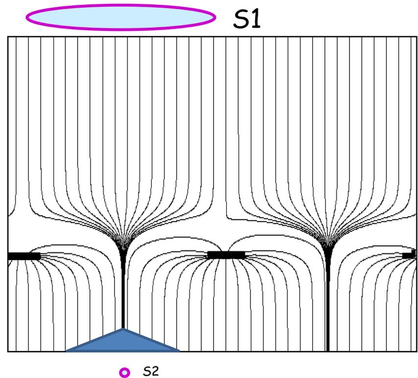
$$S2/S1 = E_{\text{drift}}/E_{\text{amplif}} \sim 200/60000 = 1/300$$
