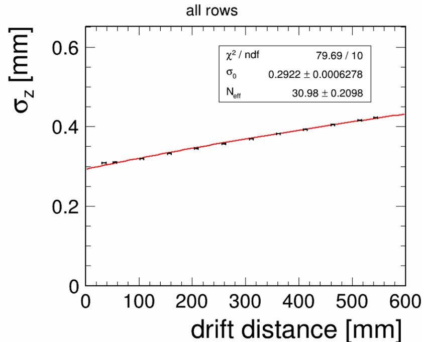
**Resolution 70  $\mu\text{m}$  in  $r\phi$  and 200  $\mu\text{m}$  in  $z$  at zero drift distance for 3mm-wide pads**
