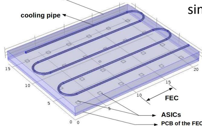
Thermal simulation of the gas volume and of the endplate modules
