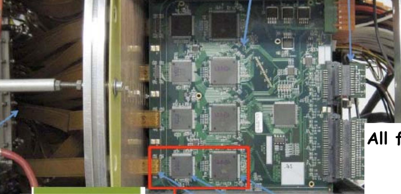
All functions are integrated into one chip: sAltro16 analog-digital mixed
