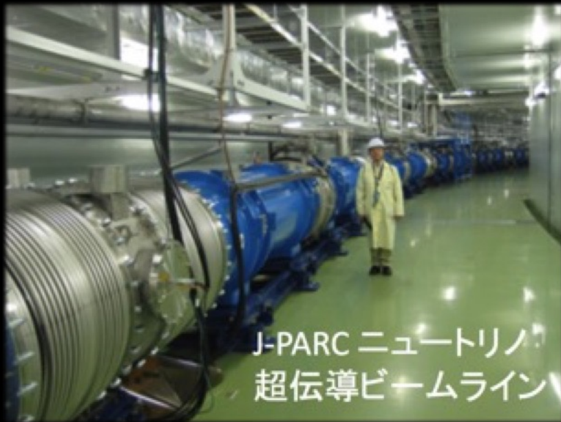
J-PARC neutrino super-conducting beam line
