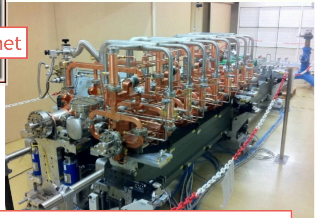
Mechanical tests of 2-beam module: active alignment and stabilisation
