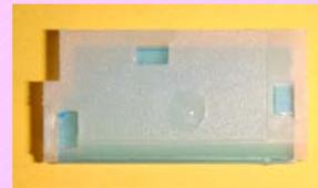
**SSBTD** (solid state nuclear detector stimulated luminescence) made of allyl diglycol carbonate ( $C_{12}H_{18}O_7$ ) which is mainly used for **neutron** detection.
