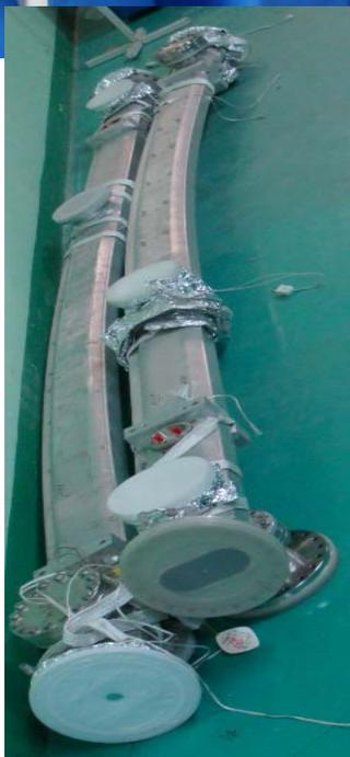
Vacuum checks have been finished , photon absorbers are installed and the supports (4 sets) for vacuum boxes are ready
