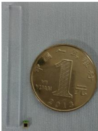
Scintillator strip and SiPM
