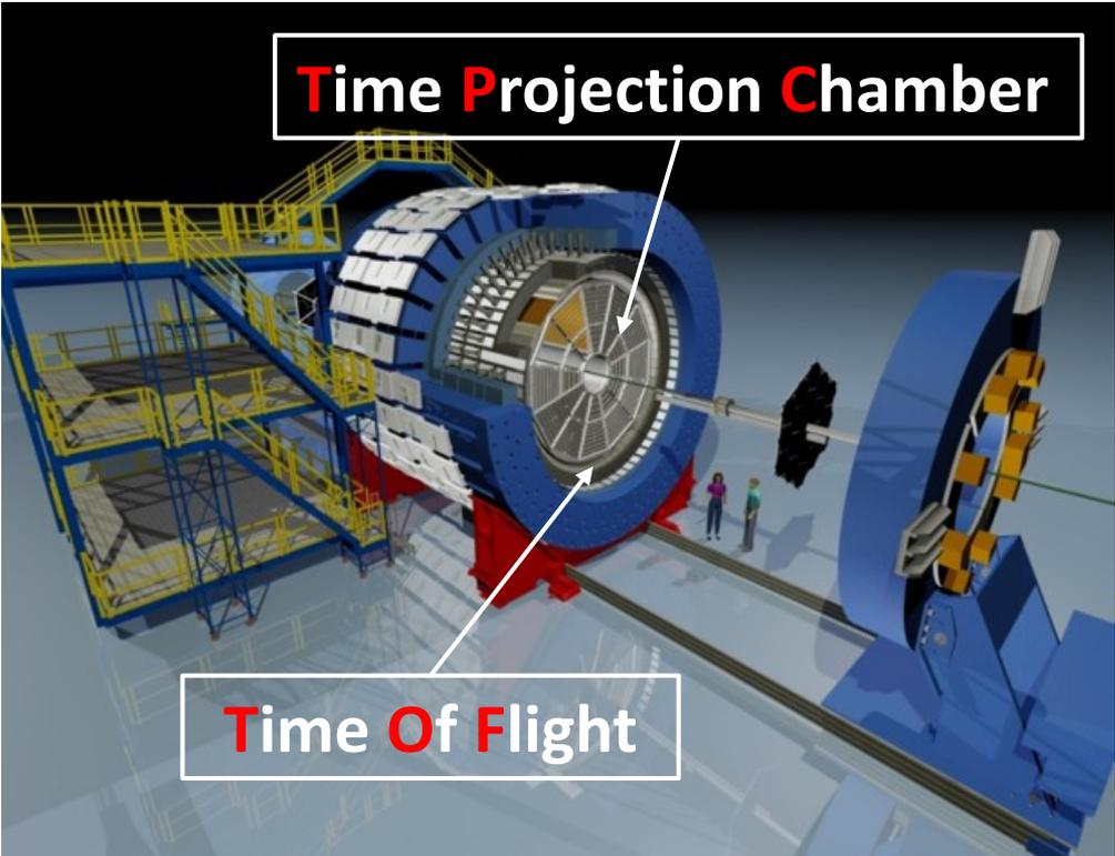
A 3D cutaway diagram of the STAR detector. The central part is a large, cylindrical Time Projection Chamber (TPC) with a grid of cathodes and anode planes. It is surrounded by other detector components, including a Time Of Flight (TOF) system. The diagram is color-coded with blue, yellow, and red. Two white boxes with black text and arrows point to the TPC and TOF regions.
