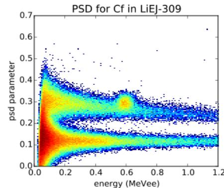
Excellent PSD performance for neutron capture & heavy recoils
