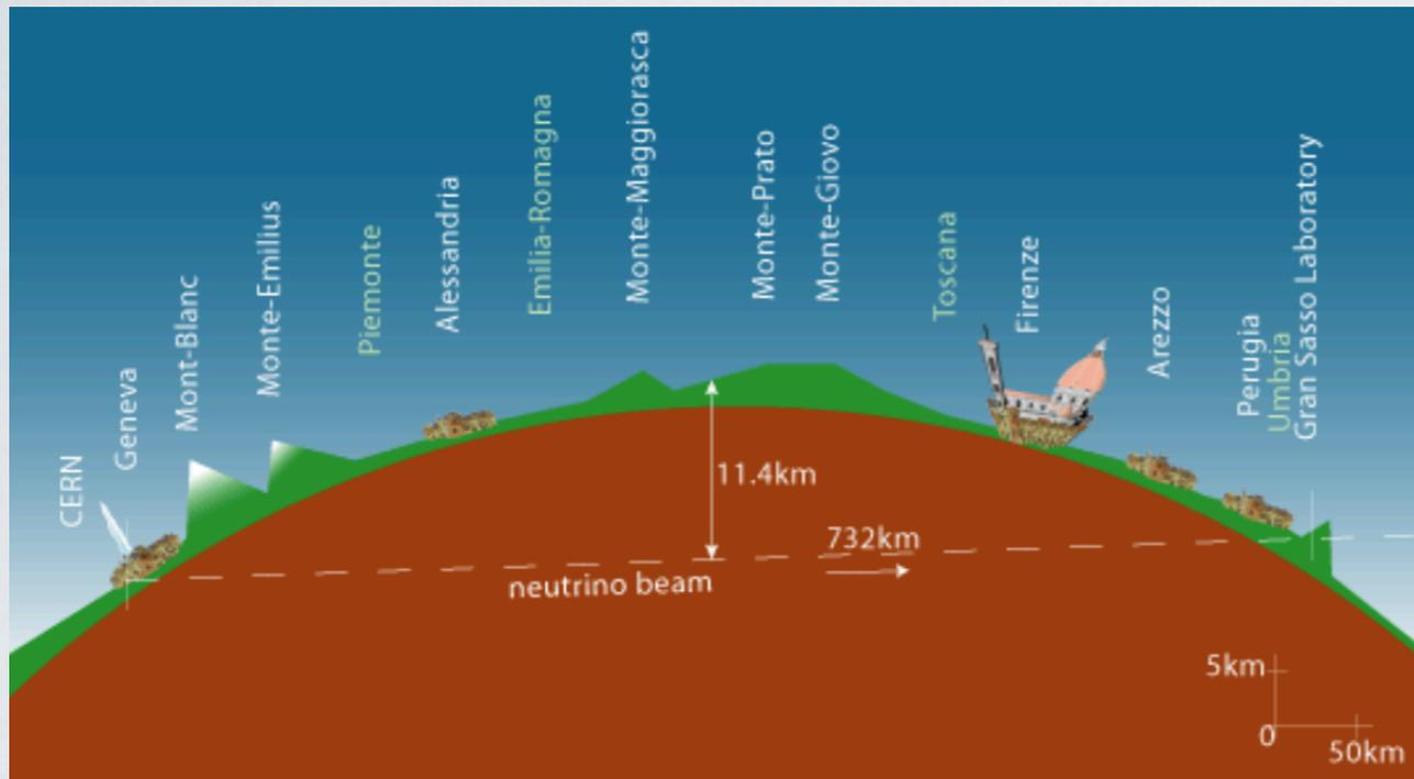
Long baseline (730 km from CERN to LNGS) neutrino oscillation experiment in the CERN Neutrino to Gran Sasso (CNGS)  $\nu_\mu$  beam
