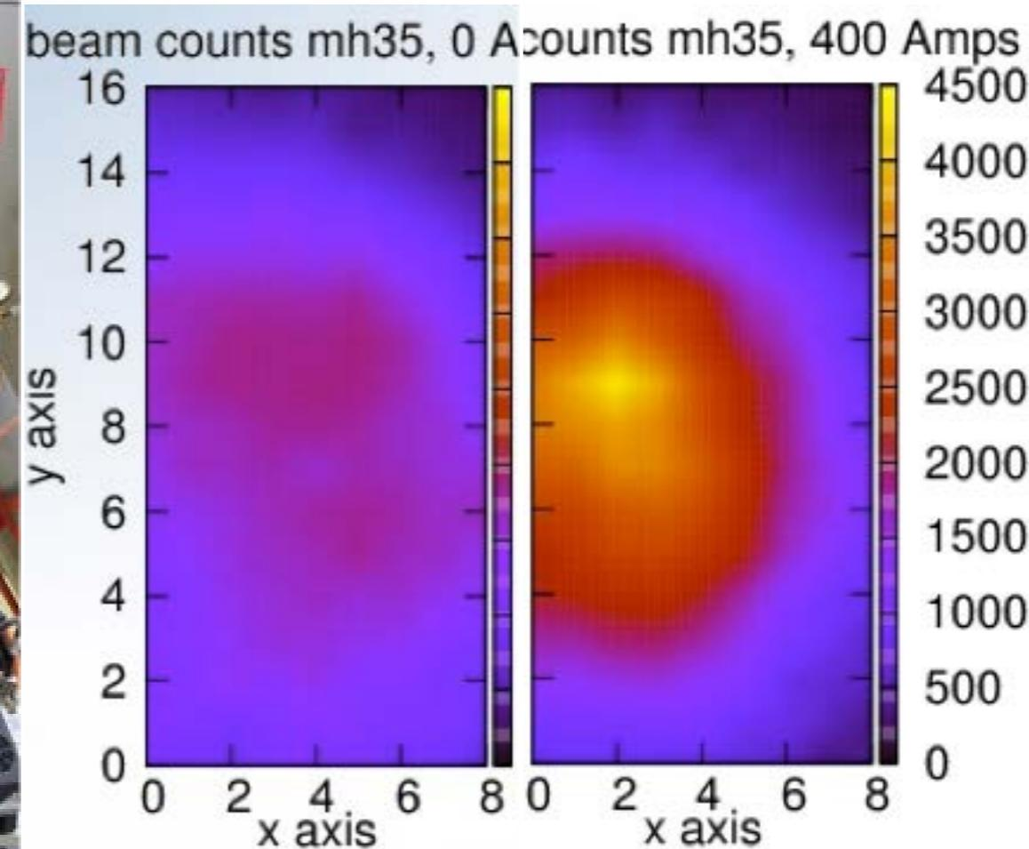
beam focusing by superconducting sextupole observed
