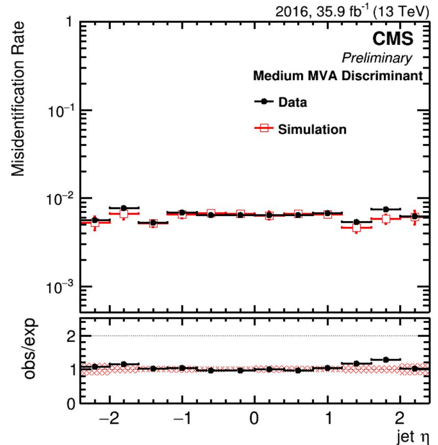
Misidentification rate of jets to taus versus p<sub>T</sub> and  $\eta$  for W+jet events after MVA medium tau identification discriminator: **average rate 0.7%** covering wide jet p<sub>T</sub> range 20 GeV - 300 GeV
