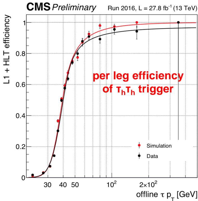
High Level Trigger efficiency of the  $\tau_h$  leg of the  $\tau_h + E_T^{\text{miss}}$  (medium isolation,  $p_T > 50$  GeV, seeded by  $E_T^{\text{miss}}$  Level-1) trigger for the  $H^\pm \rightarrow \tau_h \nu_\tau$  analysis
