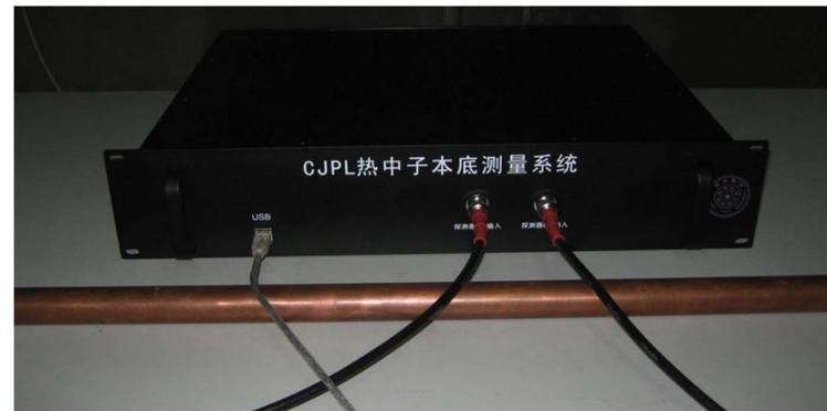
Thermal neutron measurement by He-3 tube
