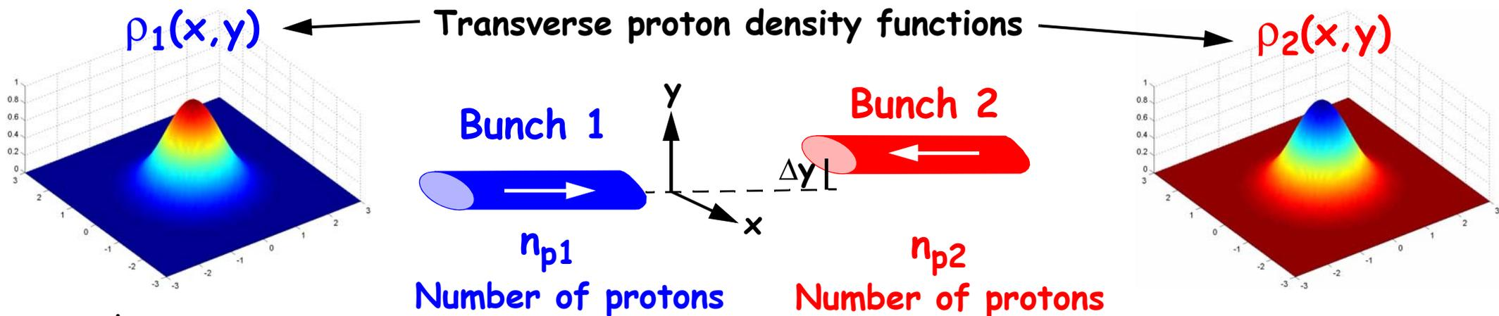
$$\mathcal{L}_{\text{Inst}}^{\text{peak}} = f_{\text{LHC}} n_{p1} n_{p2} \int \rho_1(x,y) \rho_2(x,y) dx dy$$
