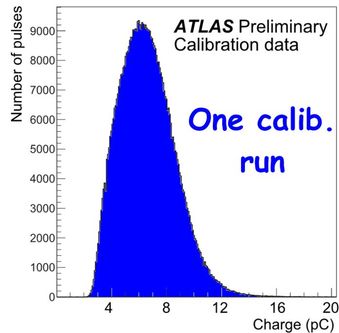
The mean values of amplitude and charge in the monitoring runs are used to correct the LUCID measurements (online & offline).
