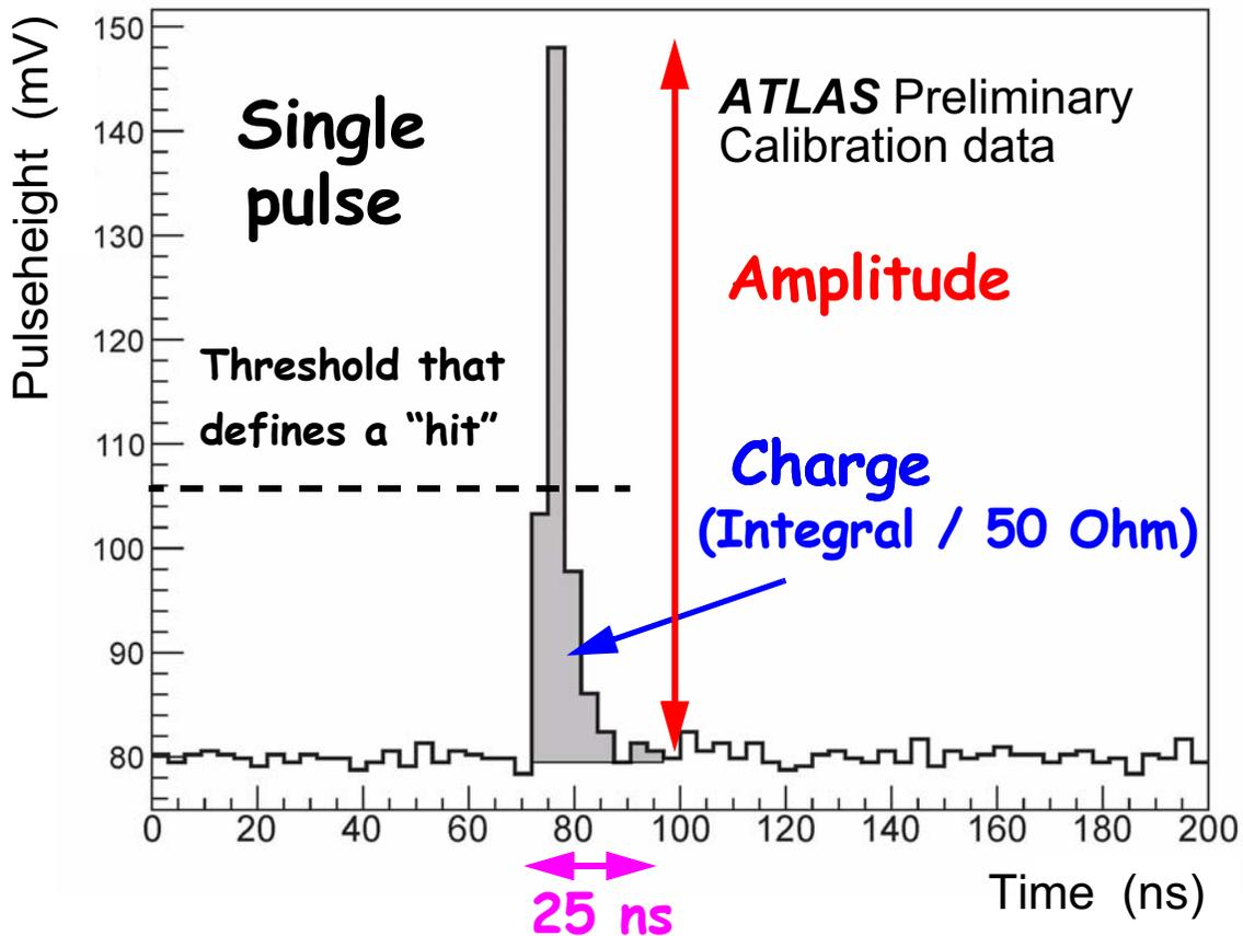
FPGAs calculate amplitude and charge in every 25 ns bunch crossing period and count hits.
