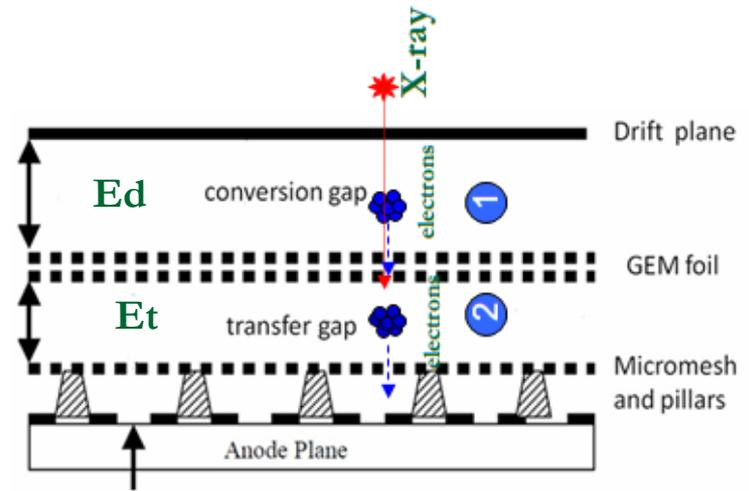
Schematic of the Gain with MM
