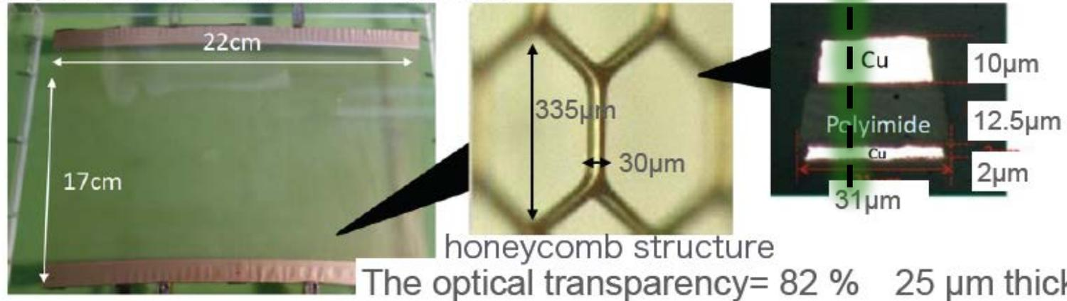
Though gating GEM stop positive ions, should not stop electron too. → Electron transmission rate is important
