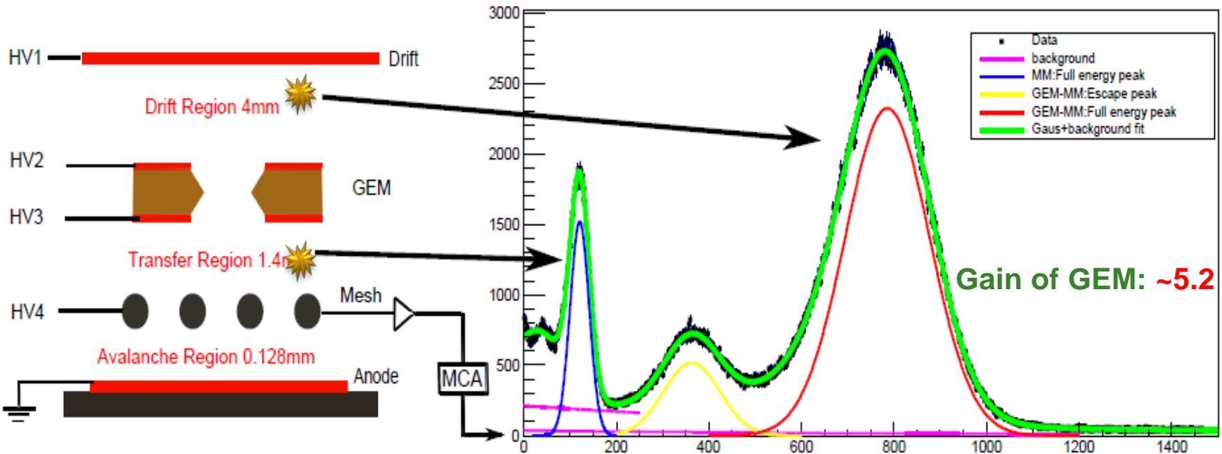
An example of the  $^{55}\text{Fe}$  spectra showing the correspondence between the location of an X-ray absorption and each peak.
