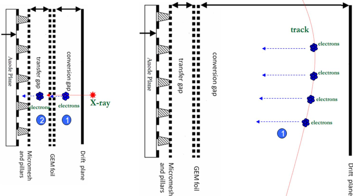
Diagram of the IBF test with the module
