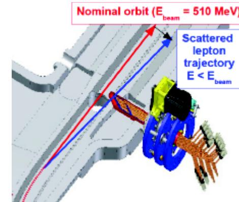
Scattered  $e^\pm$  of  $E > 400 \text{ MeV}$  escape beam pipe after first bending dipole of DAΦNE → **spectrometer**
