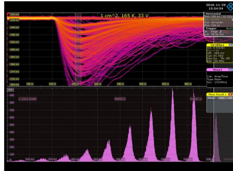
At 165 K, resolution  $\sim 0.08$  SPE r.m.s., BW 200 MHz
