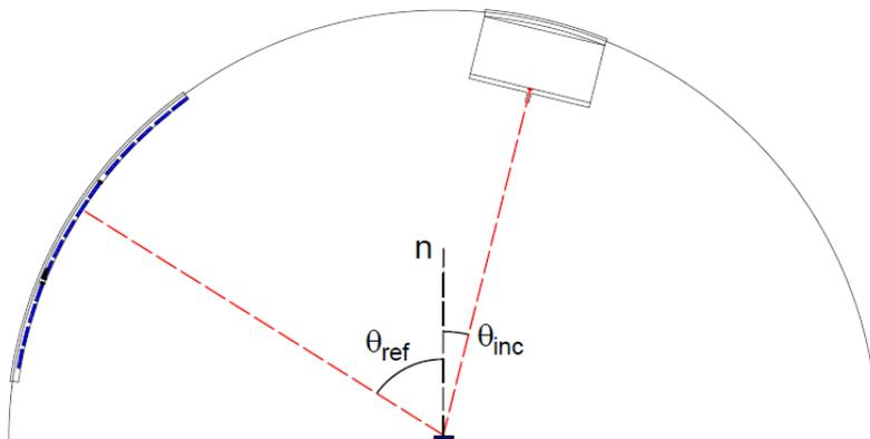
Sketch diagram of LIXO setup. Radioactive point source illuminates sample. Reflected light detected by array of SiPMs. Both source and SiPMs can slide along the rail.
