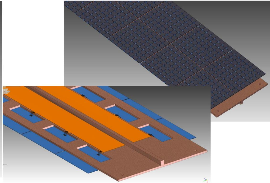
10mm x 10mm SiPMs with 0.5mm gaps, 1.5 mm gaps between tiles, 8 x 8 SiPMs per tile
