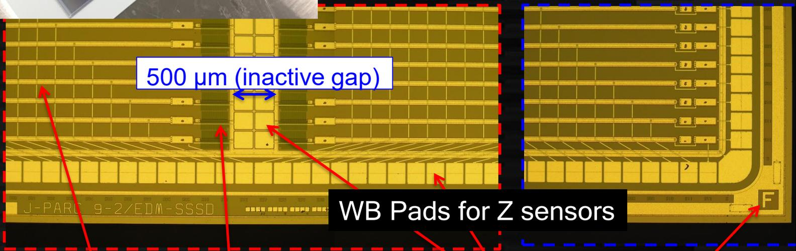
500  $\mu\text{m}$  (inactive gap)
