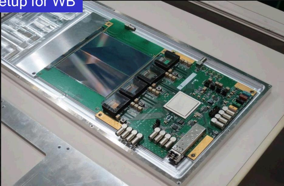
1. Fix sensor board and SliT128A multi board on mother frame on Al plate
