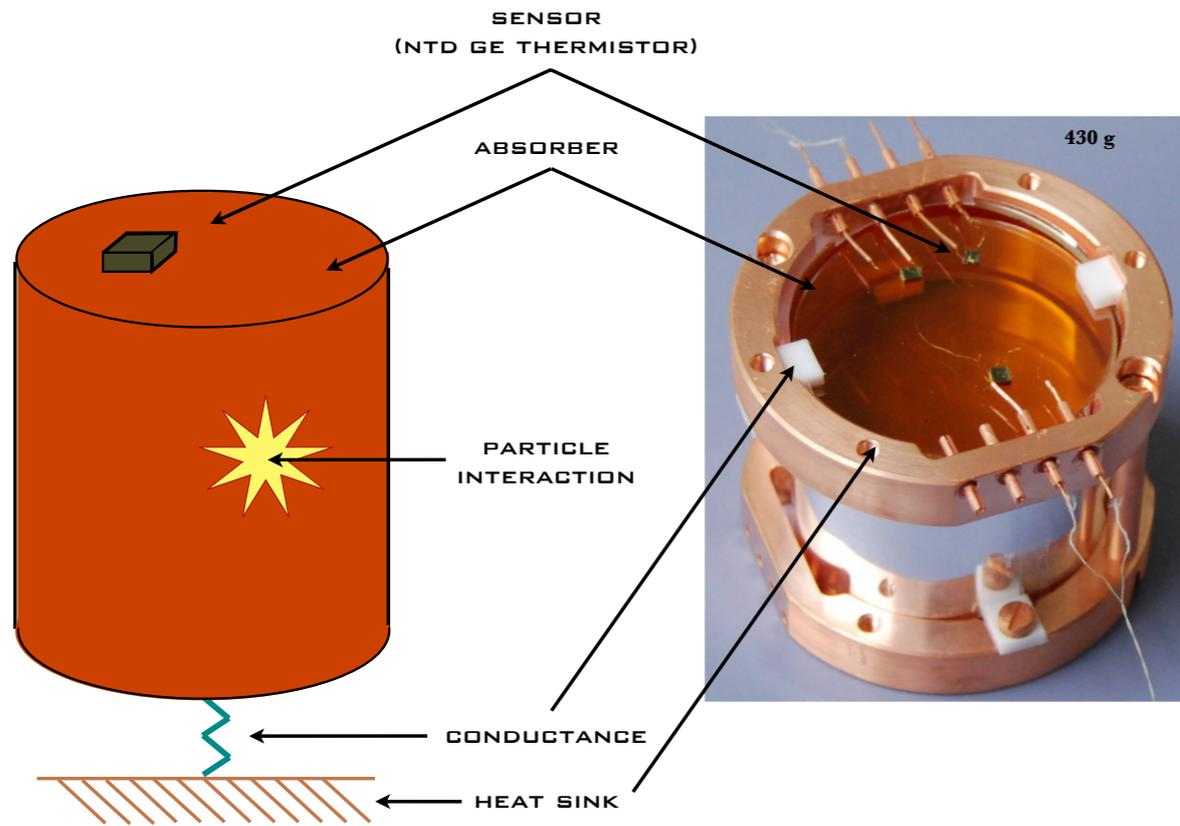
Crystal operated as calorimeter at  **$\sim 10$  mK**
