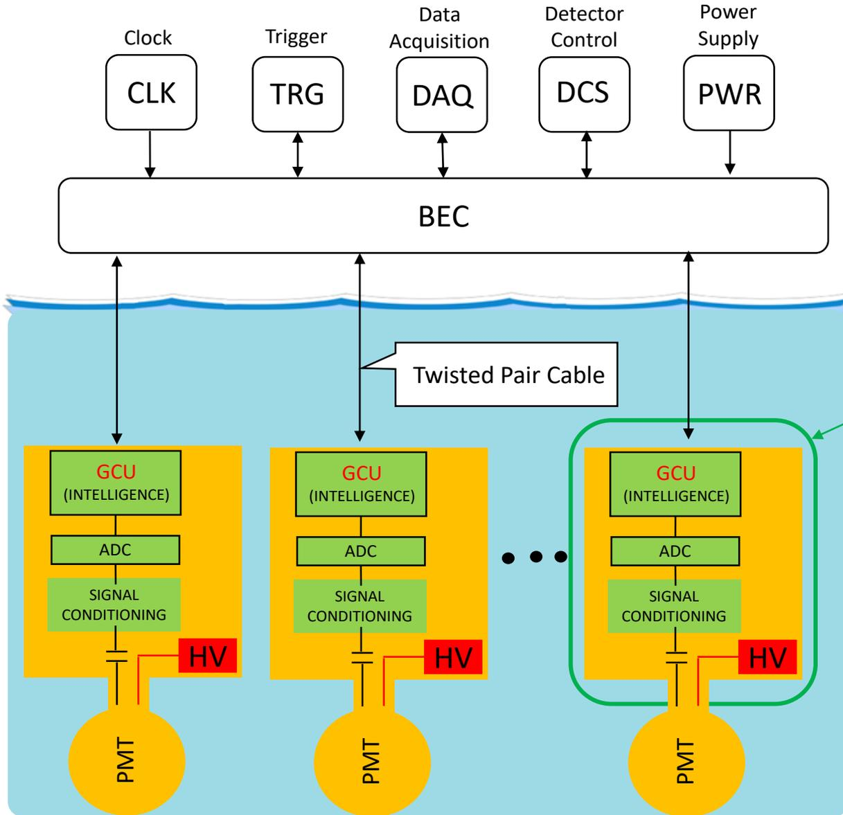
The JUNO collaboration foresees a basic readout structure in which PMT readout, trigger primitive generation, fragment buffering, baseline control, selective data readout and HV interface take place in a watertight box sealed together with the PMT. Each readout electronics box communicates with the external world via 4 pairs of copper cable CAT5e with an estimated length of  $\sim 100\text{m}$ .
