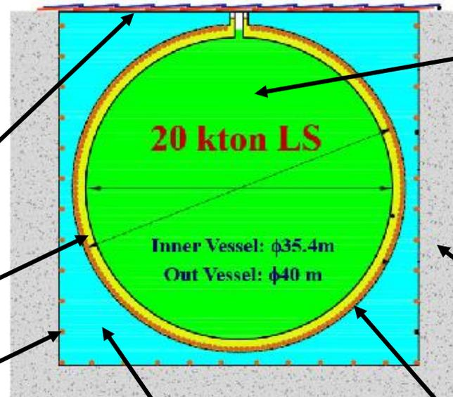
Acrylic sphere holds 20kton of scintillator liquid.
