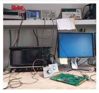
**The input signal** is made by a pulse generator signal: a negative voltage pulse (rise time= 5ns, fall time= 5ns, width= 10 ns, Amplitude @1 p.e.~ 0.8 mV).
