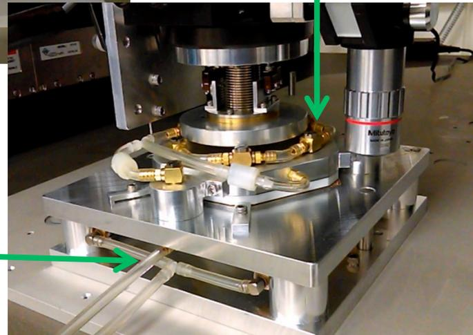
(1) Module baseplate is vacuum chucked during assembly
