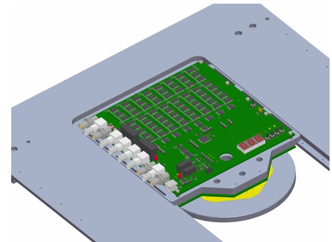
CAD drawings of the assembled cards. Pogo pins can be seen in the top picture.
