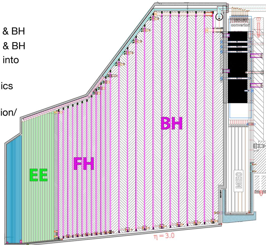
**Endcap Electromagnetic calorimeter (EE):** Si, Cu & CuW & Pb absorbers, 28 layers,  $25 X_0$  &  $\sim 1.3 \lambda$
