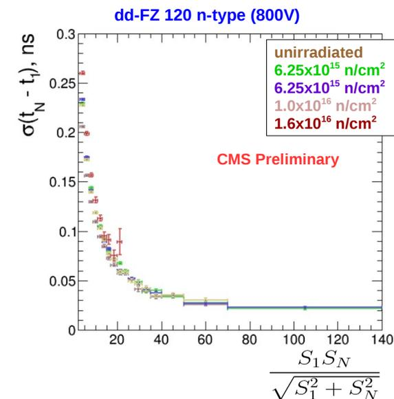
**Use thin sensors in the inner most layers, operate cold and at higher voltage.**
