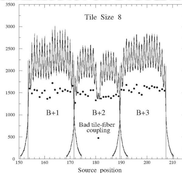
FIGURE 5. The PMT current as a function of the source position for three adjacent cells.
