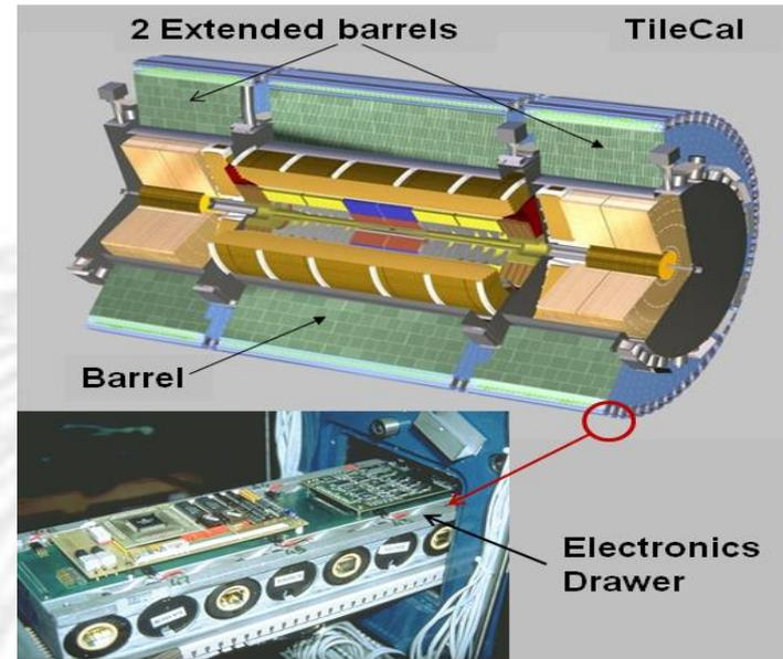
Measure light produced by charged particles in plastic scintillator.
