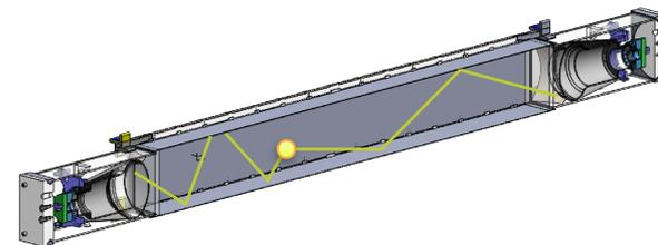
The scintillation light generated is constrained in the cell and detected by the PMTs, which enables event position reconstruction by timing and light difference.
