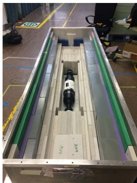
Shielded 2L prototype measuring the background
