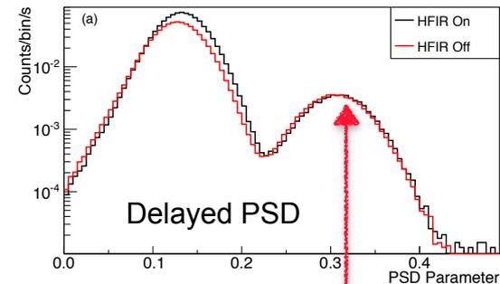
The neutron event rate between reactor on/off shows reactor correlated neutron is eliminated.
