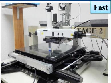
Automated scanning stage resolution ~200 nm
