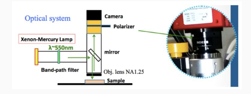
Optical microscopes have been equipped with a polarization filter. The polarization direction can be changed by rotating the polariser. The rotation is at the moment done by hand while its automation is being designed.
