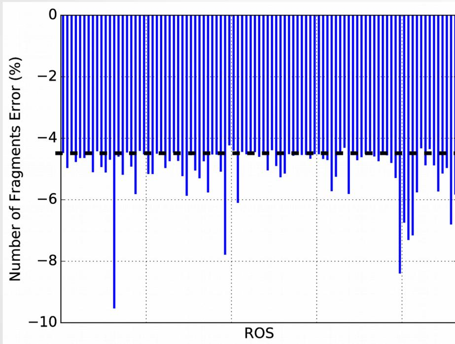
Difference (in %) between simulation and real data for the number of fragments in ROS buffers. Each bin in the plot represents a separate ROS computer, there are ~100 ROS computers
