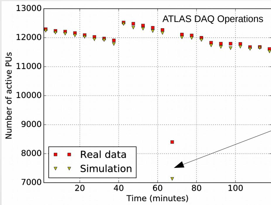
Each point in the plot represents one simulation. There are 24 simulations covering 2 hours of data.
