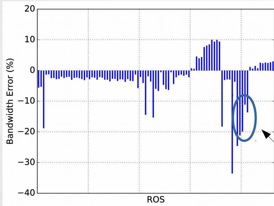
Difference (in %) between real data and simulation results for ROS output bandwidth. Each bin in the plot represents a separate ROS computer, there are ~100 ROS computers
