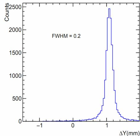
Apparent transverse shift of sensors with linear dependence on longitudinal position: most likely explained by relative inclination of the beam direction.
