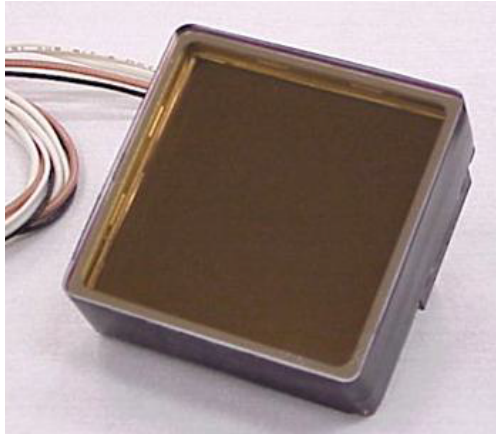
Photonis Planacon 53mm x 53mm, 8x8 25 \mu\text{m} pore, L/d = 40
