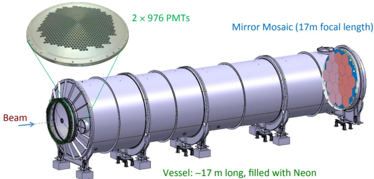
Neon gas slightly above atmospheric pressure
