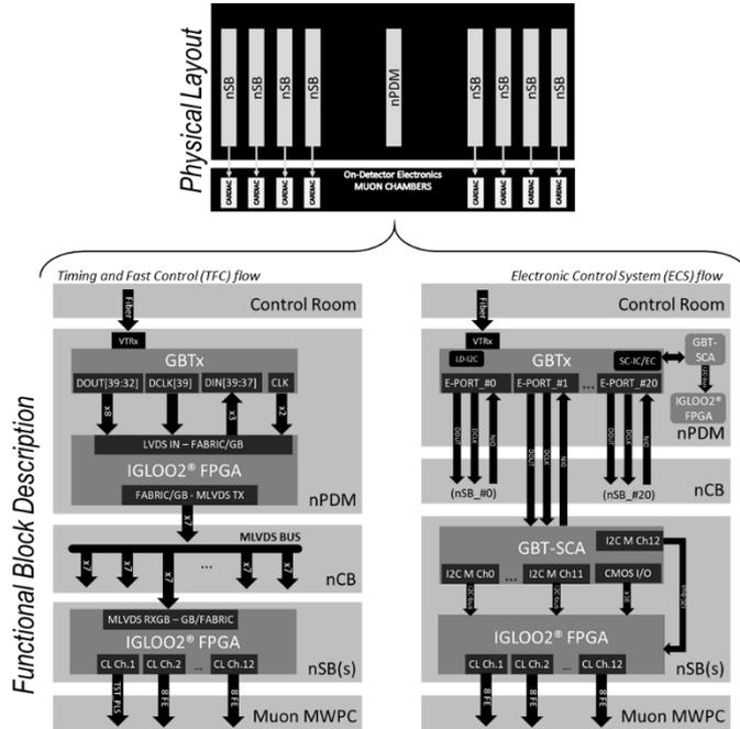
**Fig. 1.** Quick Physical and Functional overview of the new Service Board System.
