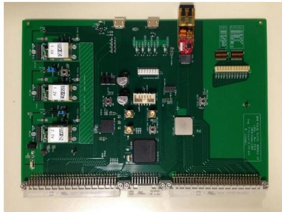
**Fig. 4.** The new Pulse Distribution Module (nPDM) prototype rev.01, produced in March 2017
