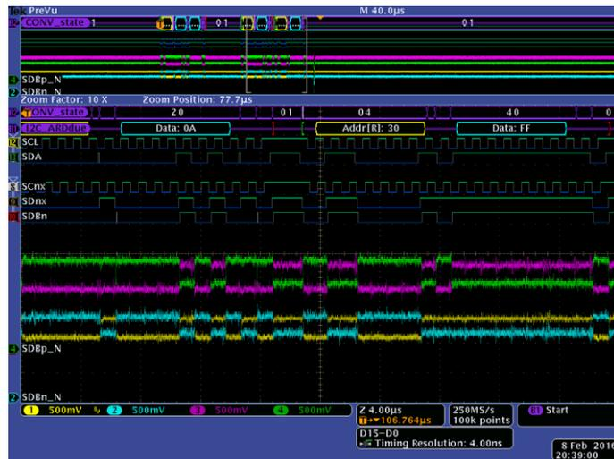
**Fig. 2.** Screenshot of two successful I2C transaction (W and R) between a commercial I2C driver (SCL/SDA) and the muon On-Detector Electronics custom serial link (SCNx/SDNx/SDBn).
