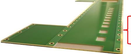
Shield protects analog circuits from digital noise from front AMC backpane
