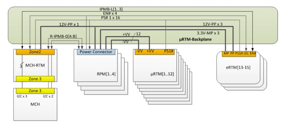
Greatly increased Analog via rear ±V power options, total AMC+RPM power, extension of control to additional crates
