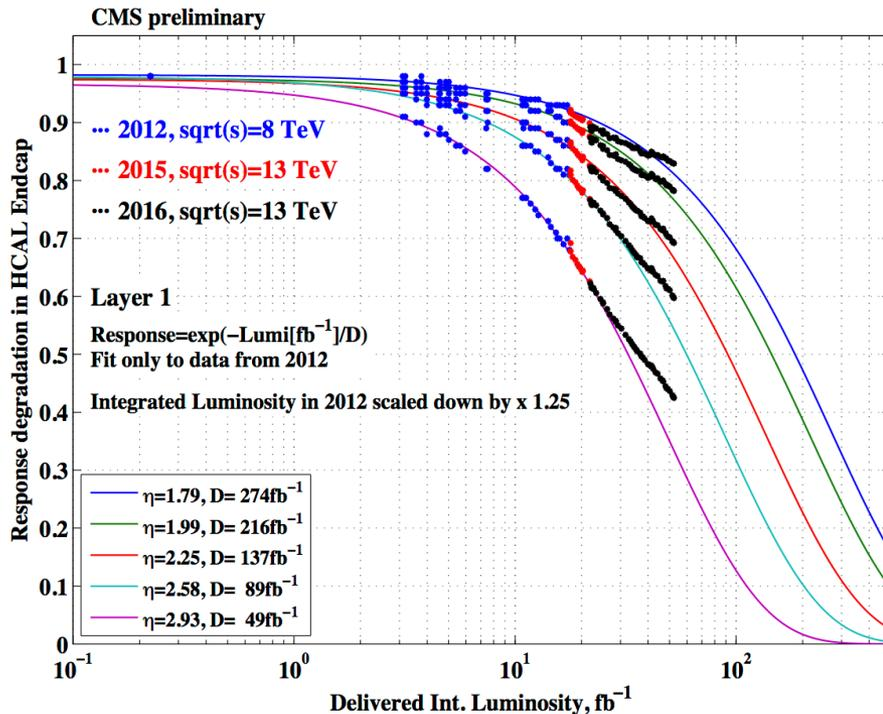
The dependence of the radiation damage on the rate at which the radiation dose is delivered is well (re-) established
