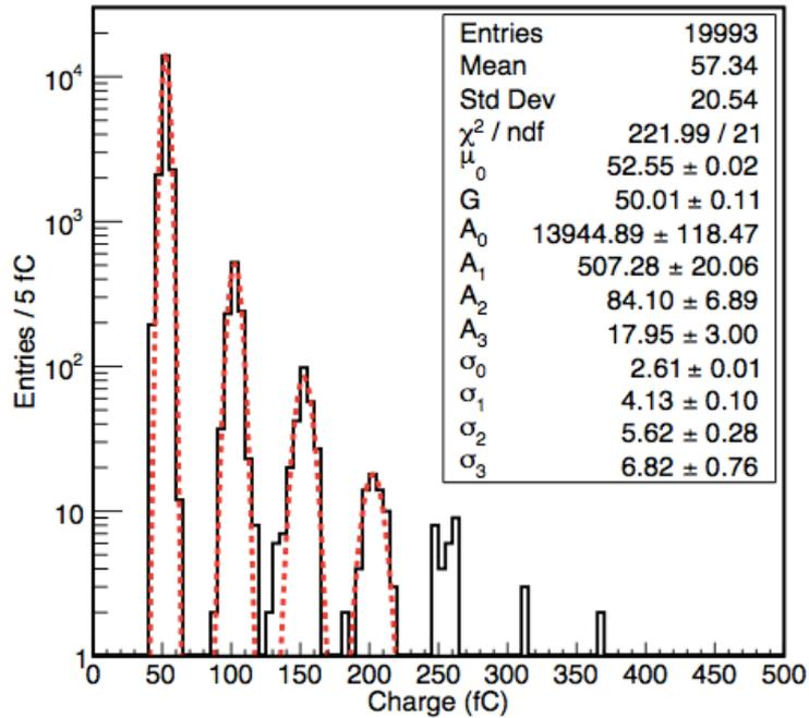
Single fit function for the entire spectrum down to three orders of magnitude drop of the peak.
