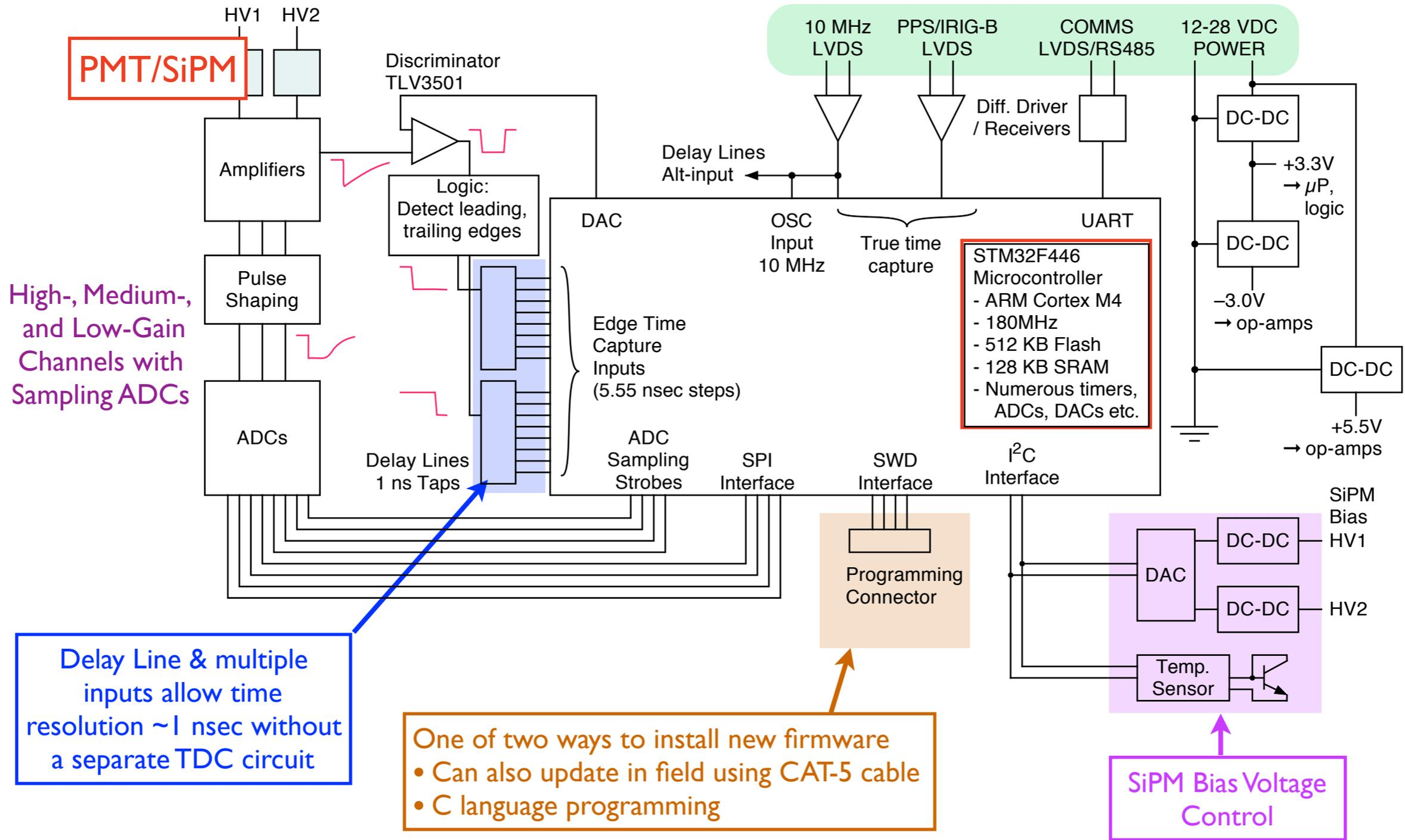
Delay Line & multiple inputs allow time resolution ~1 nsec without a separate TDC circuit
