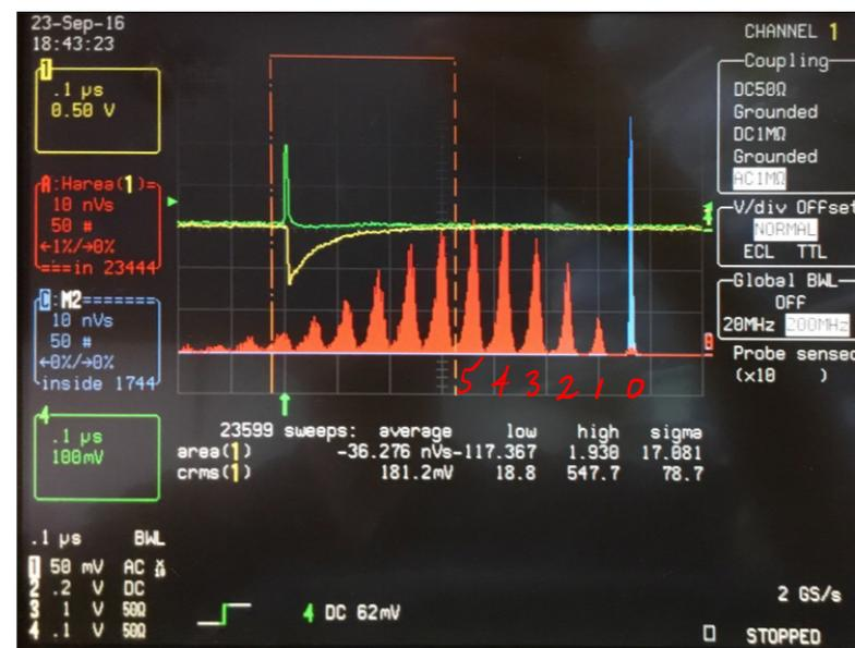
SiPM+  $\mu$ DAQ charge spectrum
