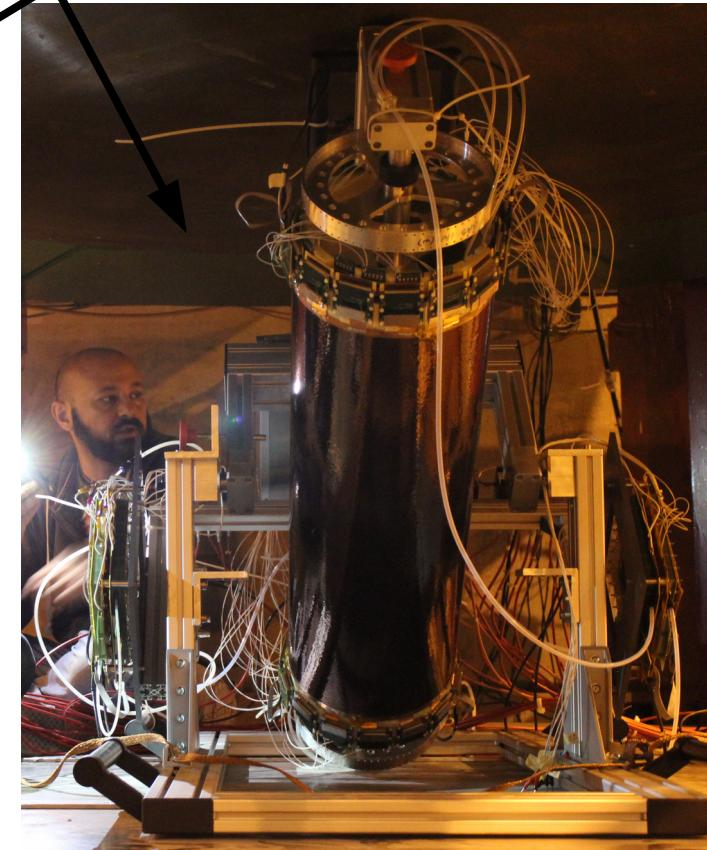
The aim of the cosmics run and the TB is to measure the performance of the CGEM and to compare it with the results obtained with the planar GEM
