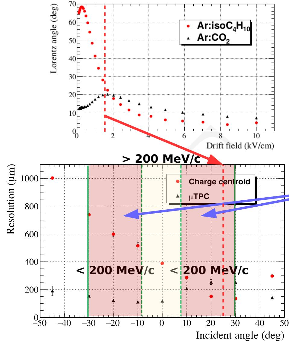
Expected entrance angle at the outer radius of CGEM-IT (primary vertex particles)
