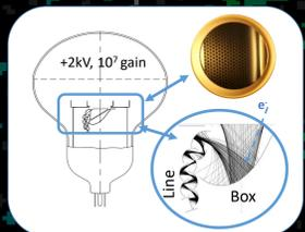
**Box & Line type PMT (50 cm Ø)**
