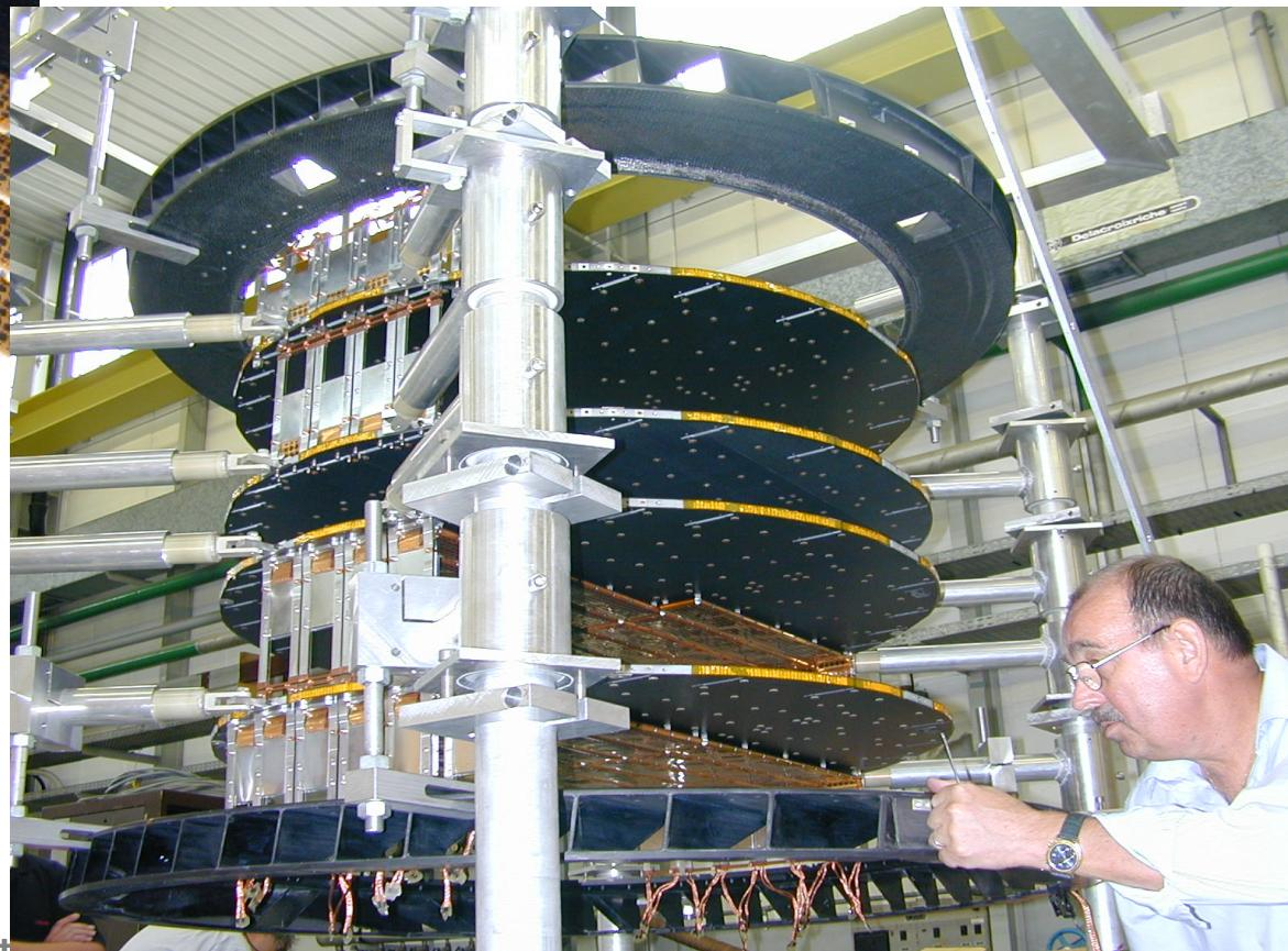
Lightweight carbon fiber shell to hold the planes
