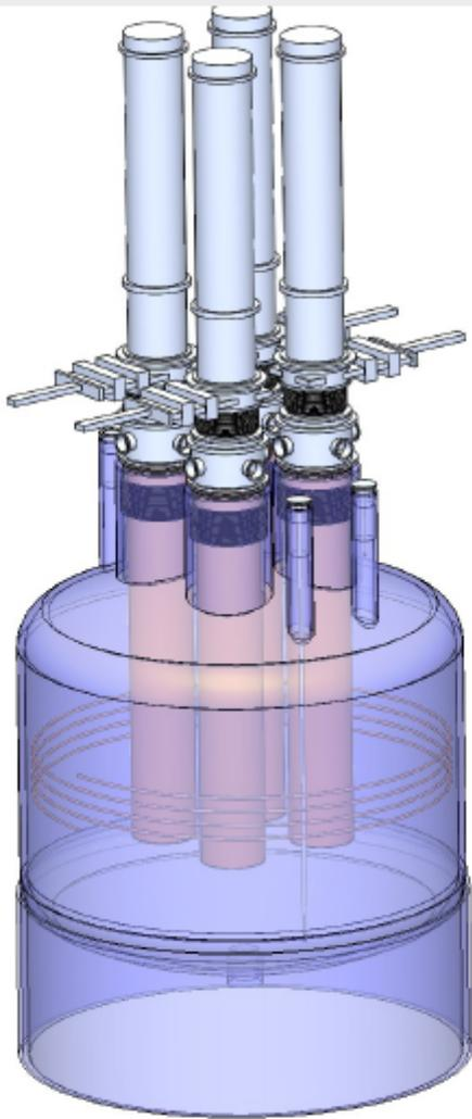
cryostat sketch for 4x250 kg
