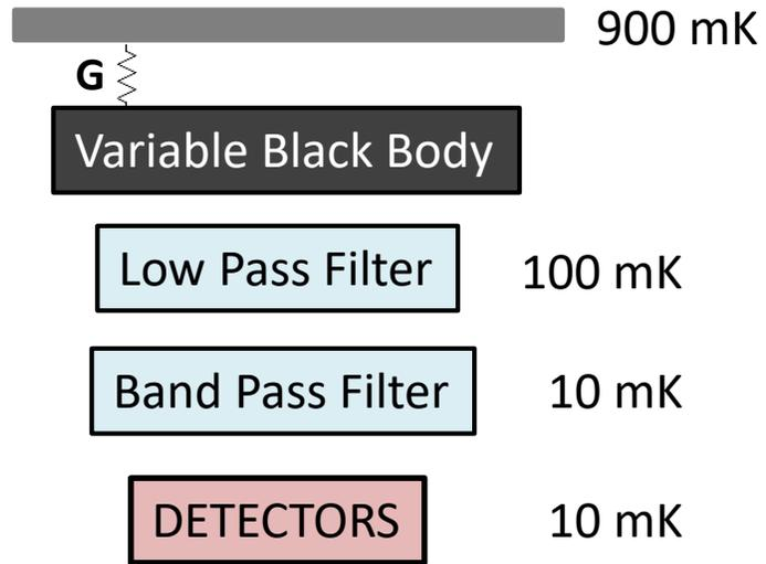
We realized a test-bed to simulate mm-wave optical signals in low-background conditions
