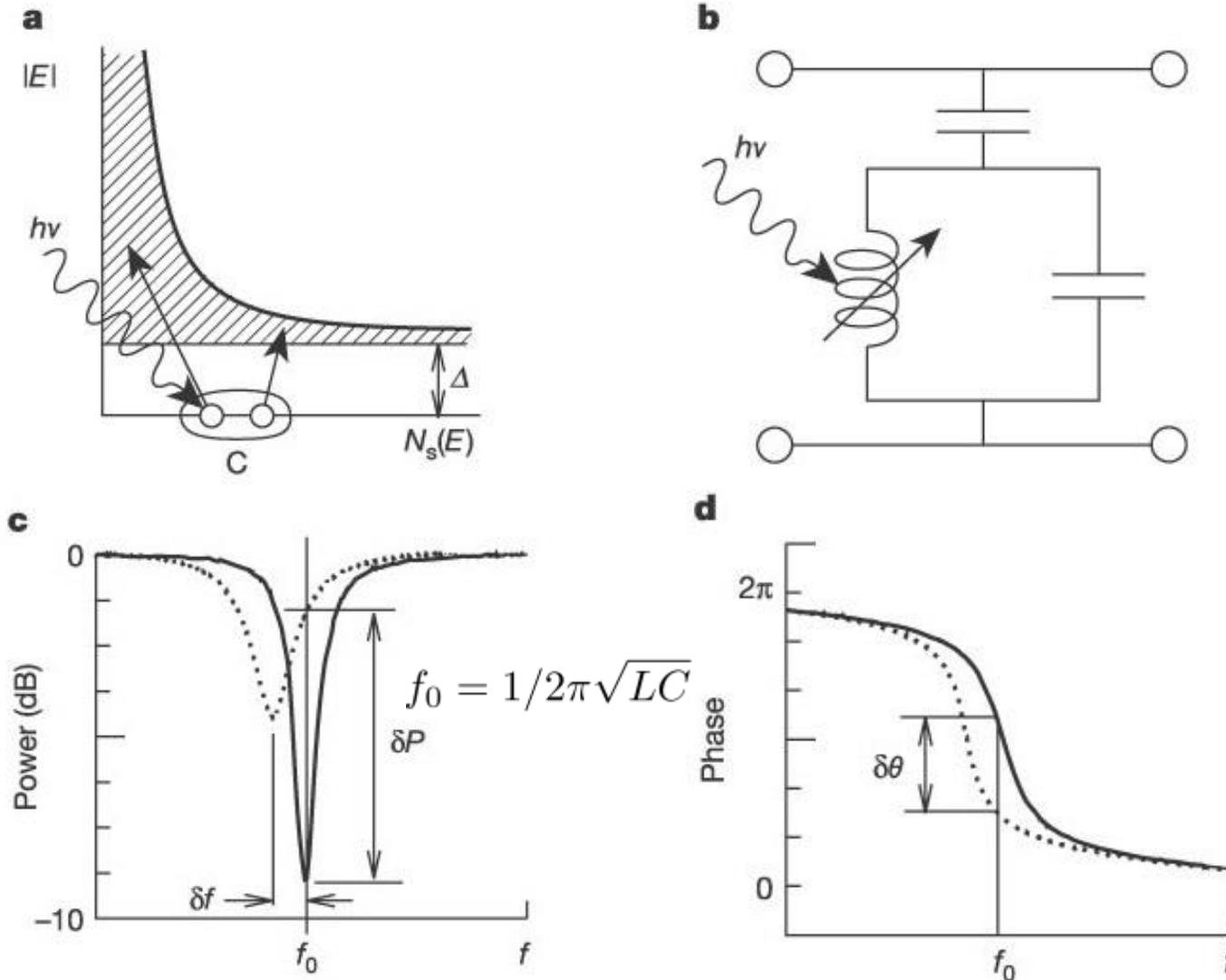
Cooper pairs (CP) in a superconductor act as an inductance ( $L$ ). Absorbed photons change cp density and  $L$ .
