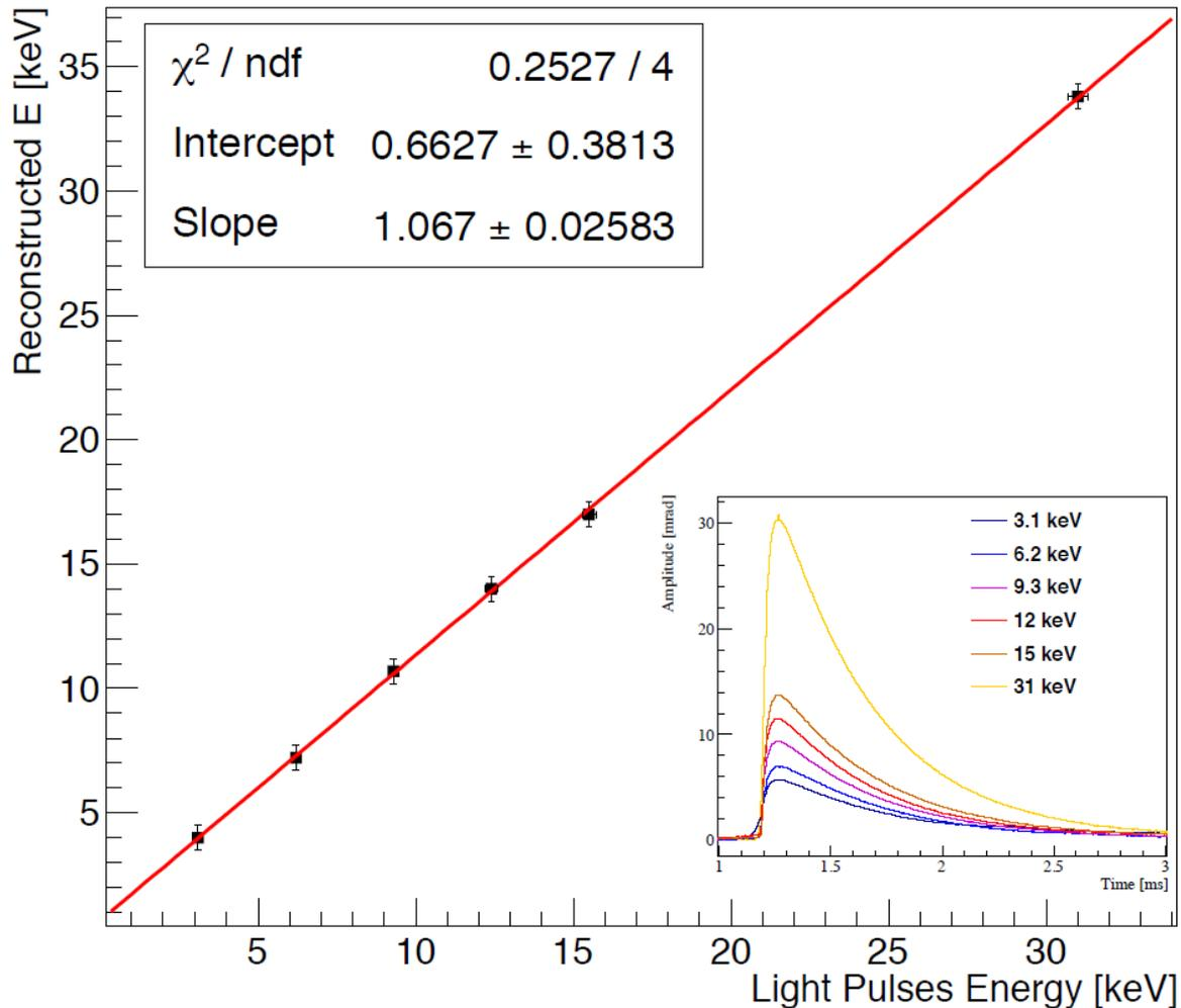
Detectors are illuminated using a 400 nm fast LED at 293 K, coupled with an optical fiber.
