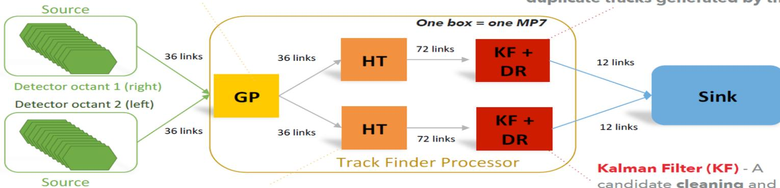
**Hough Transform (HT)** - A highly parallelised first stage track-finder that identifies groups of stubs consistent with a track in the  $r-\phi$  plane
