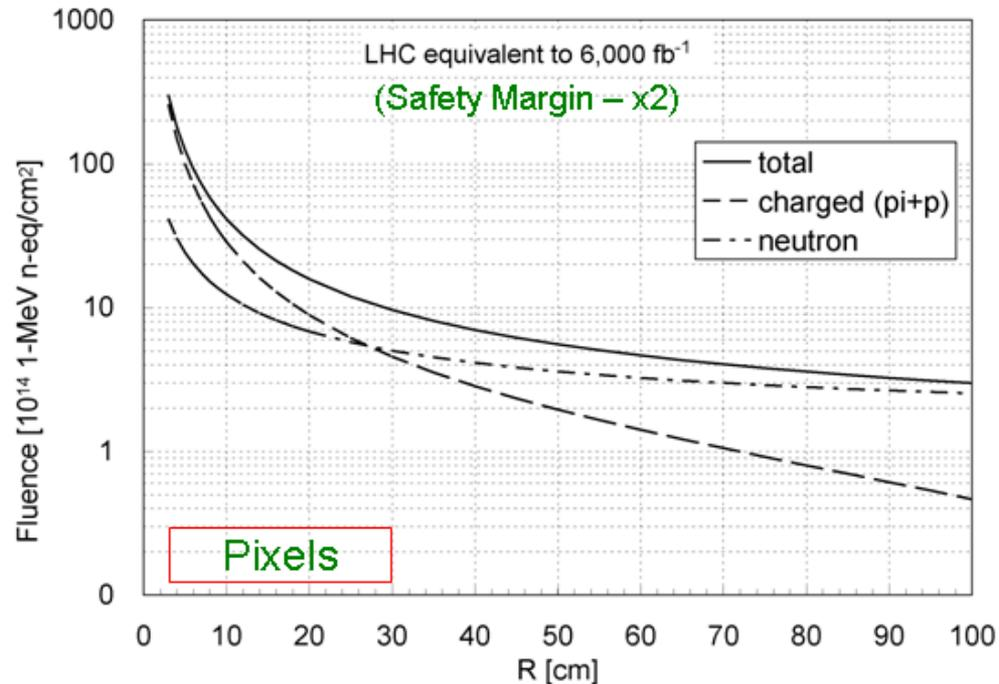
Radiation Tolerance Scale of inner layers is  $10^{16}-10^{17}\text{cm}^{-2}$  ( $>500\text{Mrad}$ )
