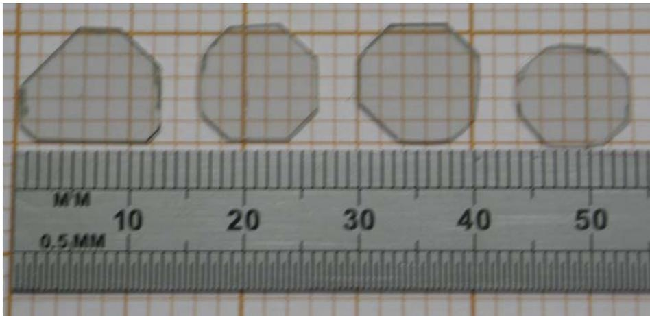
Wafers 5-10mm  $\times$  5-10mm; scCVD diamond collects full charge
