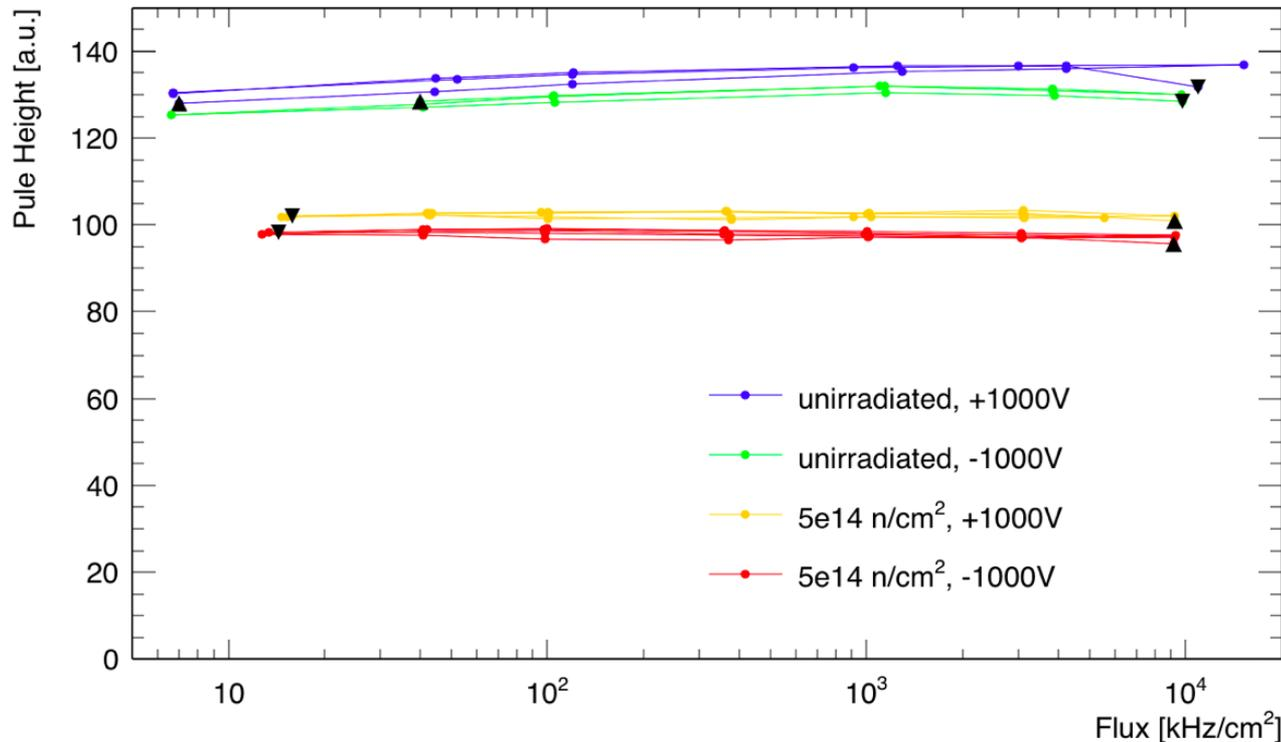
No rate dependence observed in pCVD up to 10-20MHz/cm<sup>2</sup>
