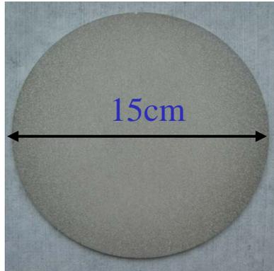
Wafers 15cm diameter; wafer collection distance  $400\mu\text{m}$ - $500\mu\text{m}$
