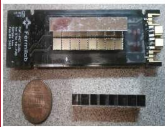
8x2 LYSO crystals/SiPMs read by using 2 strip lines
