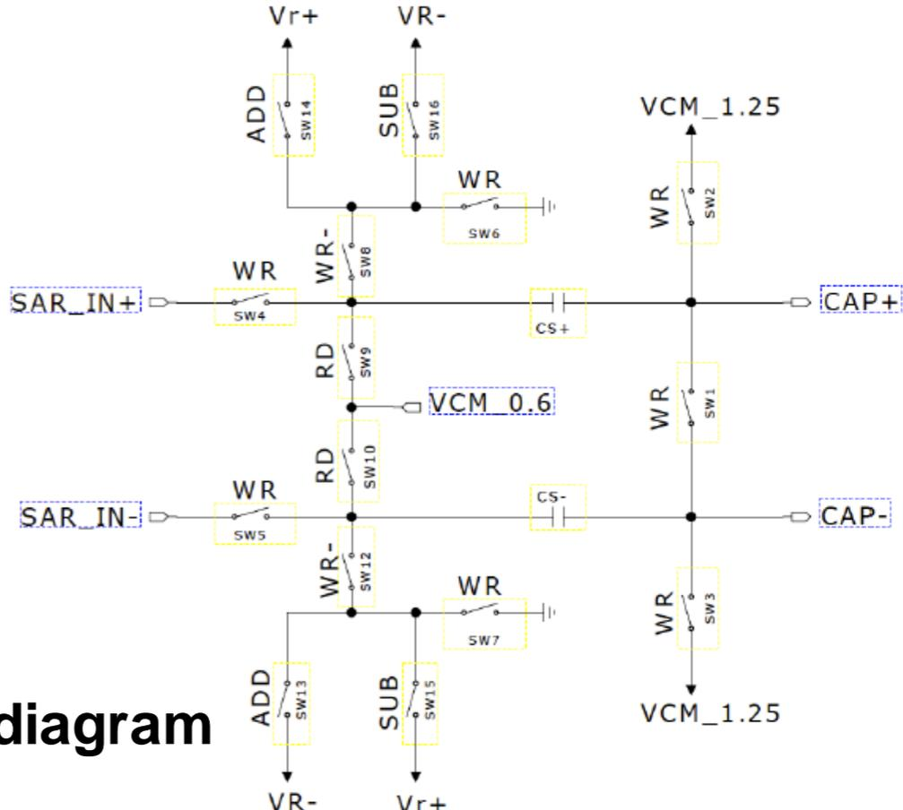
SAR switch schematic diagram
