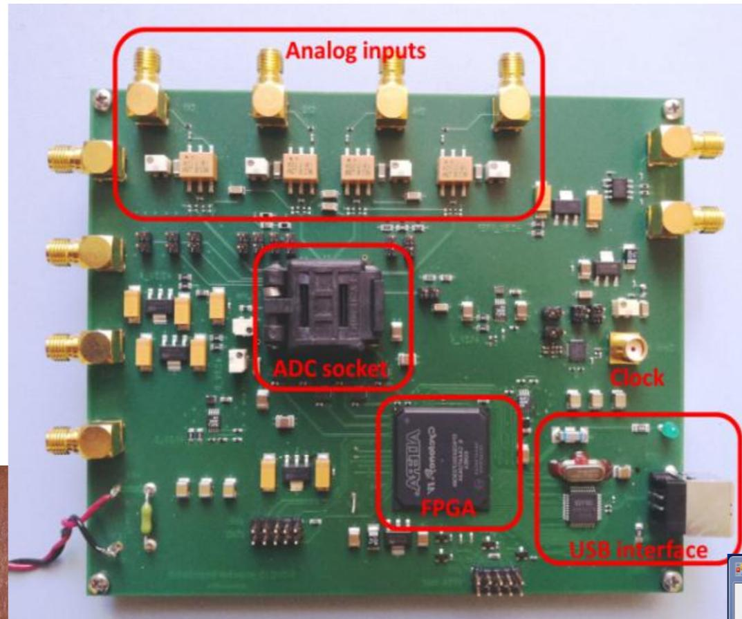
ADC test socket board
