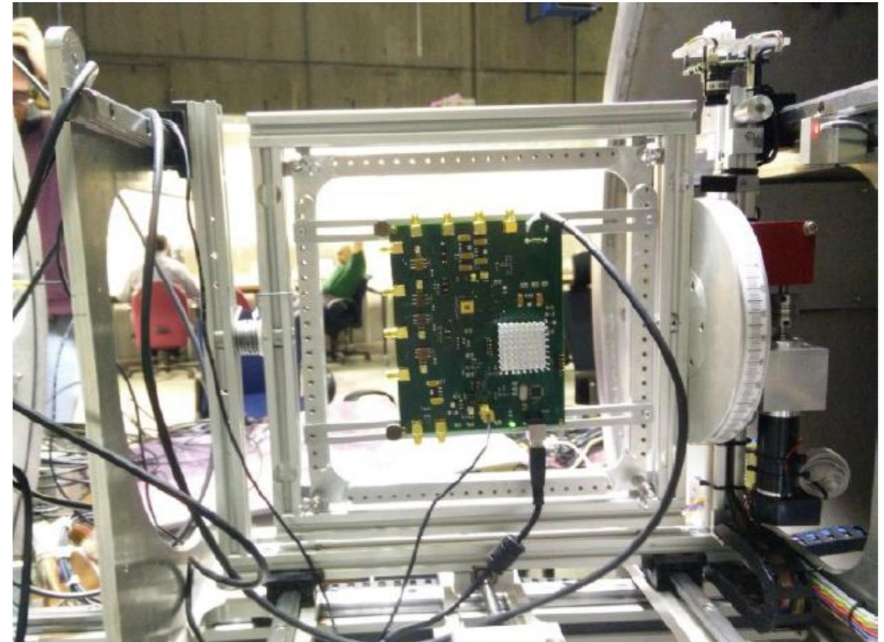
**Fig. UC Louvain's cyclotron using heavy ions with open lid package**
