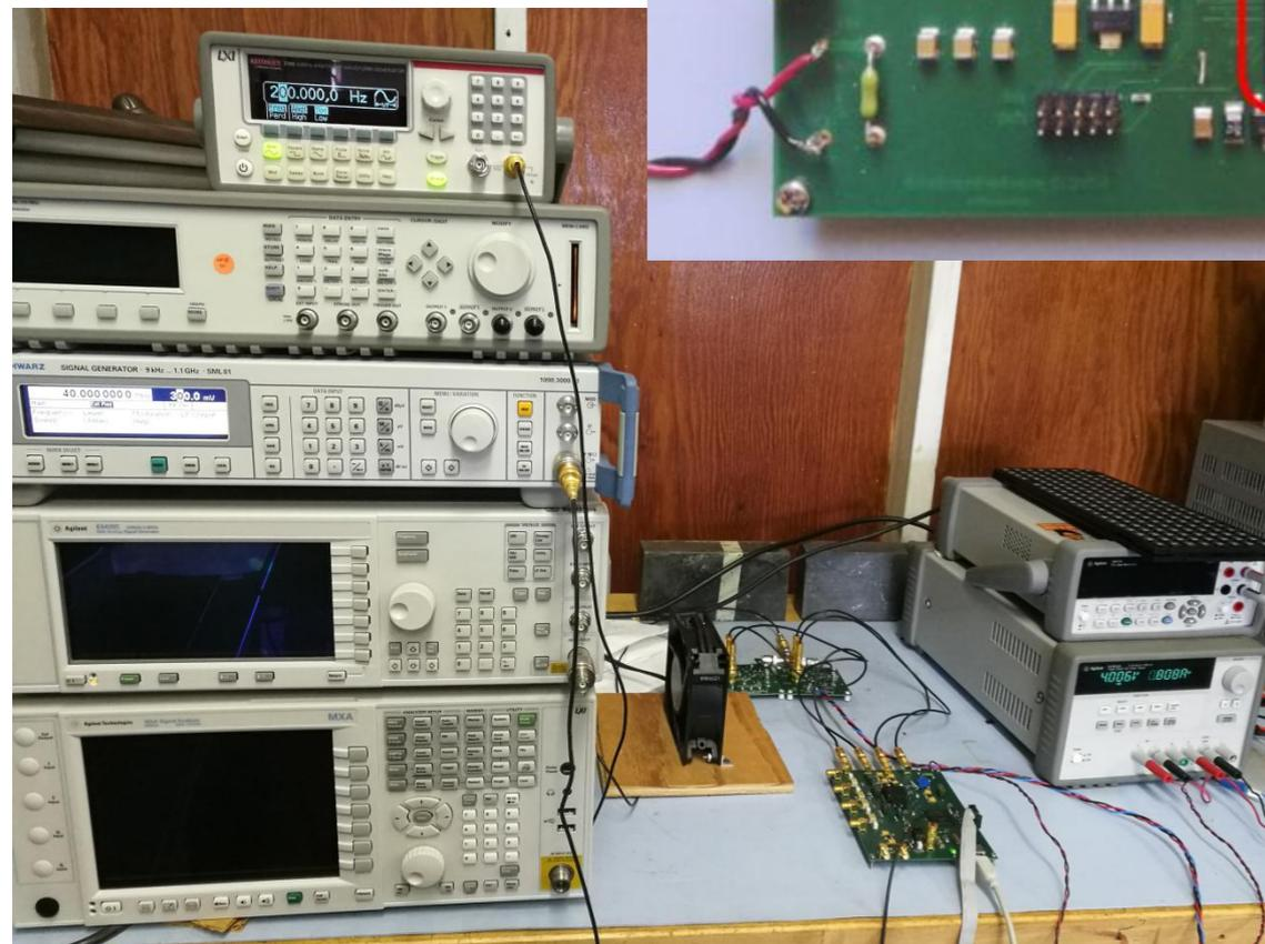
ADC test setup
