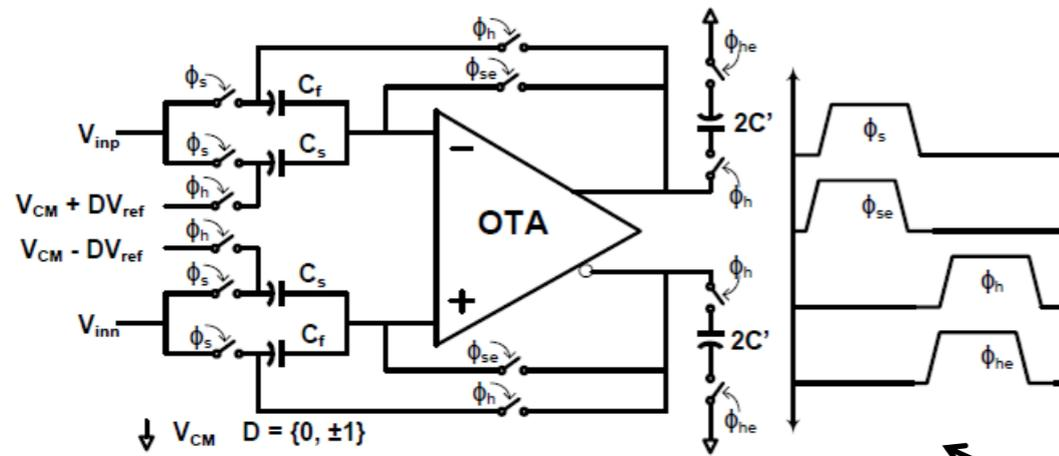
$$V_{out} = 2 * V_{in} - D * V_{ref}$$
