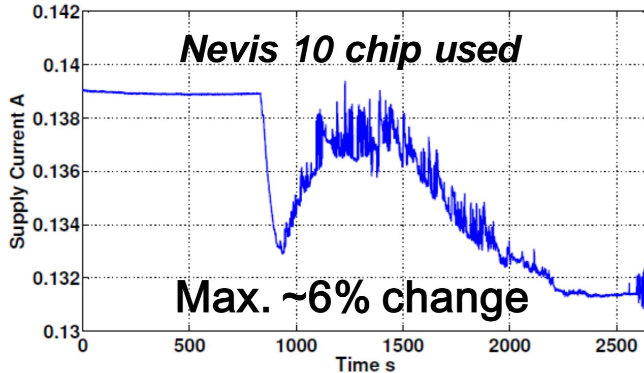
Fig. Current consumption change during irradiation. (2500 s horizontal scale corresponds to a dose of 5 Mrad)
