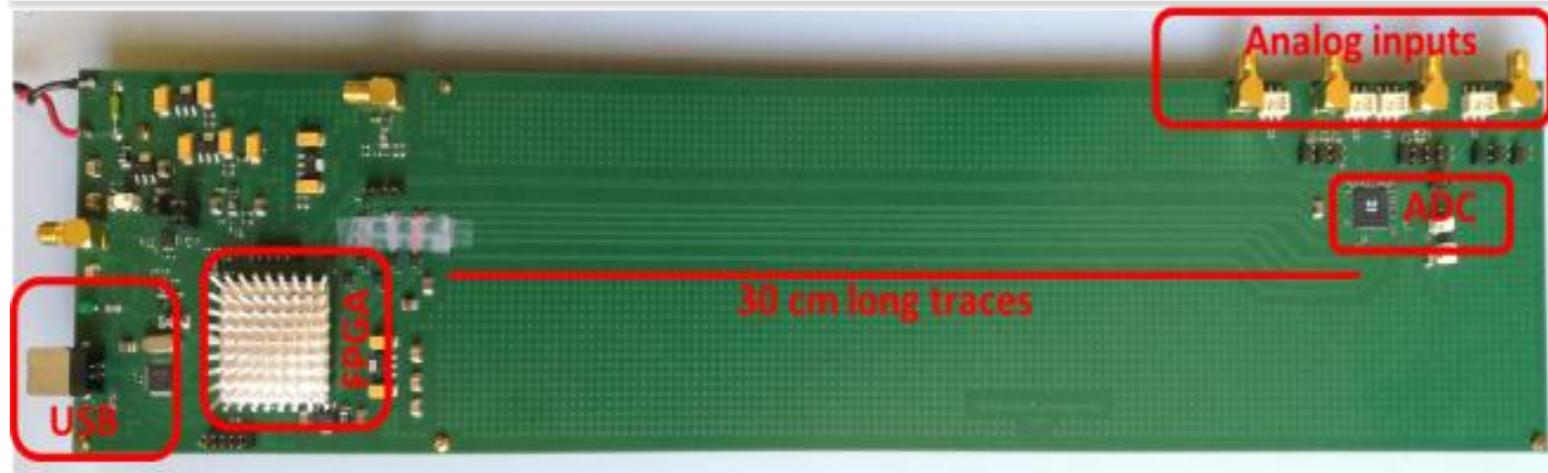
**Fig. Long radiation tester board**
