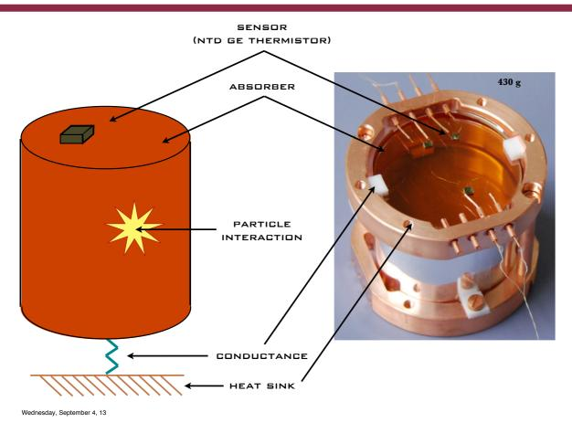
Crystal operated as calorimeter at ~10 mK Particle interaction  $\Rightarrow$  E deposit  $\Rightarrow$  T increase Dedicated sensor to convert  $\Delta$ T in a voltage pulse
