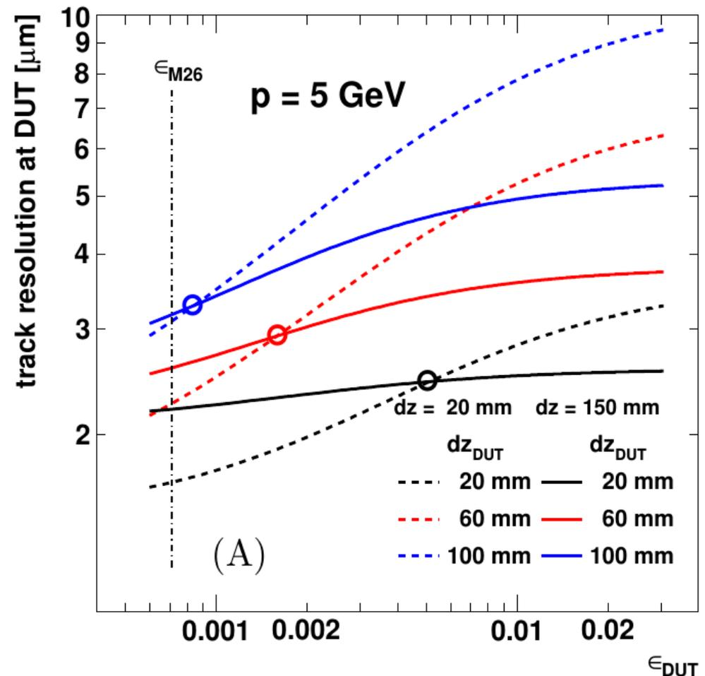
→ Thick DUT: use wide set-up
