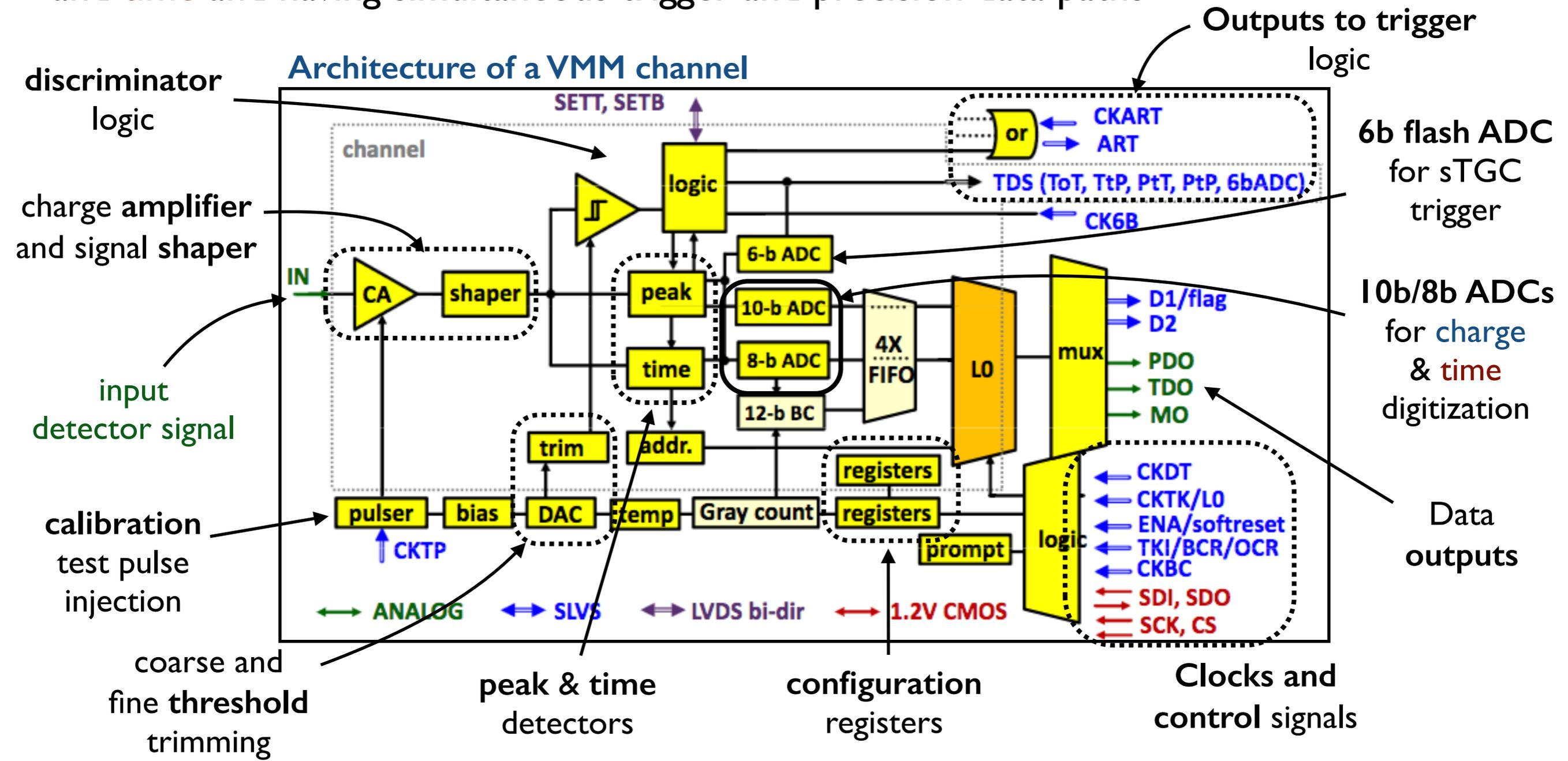
**512 Mb/s (8b/10b) output capability, giving a max 5MHz hit rate per channel**
