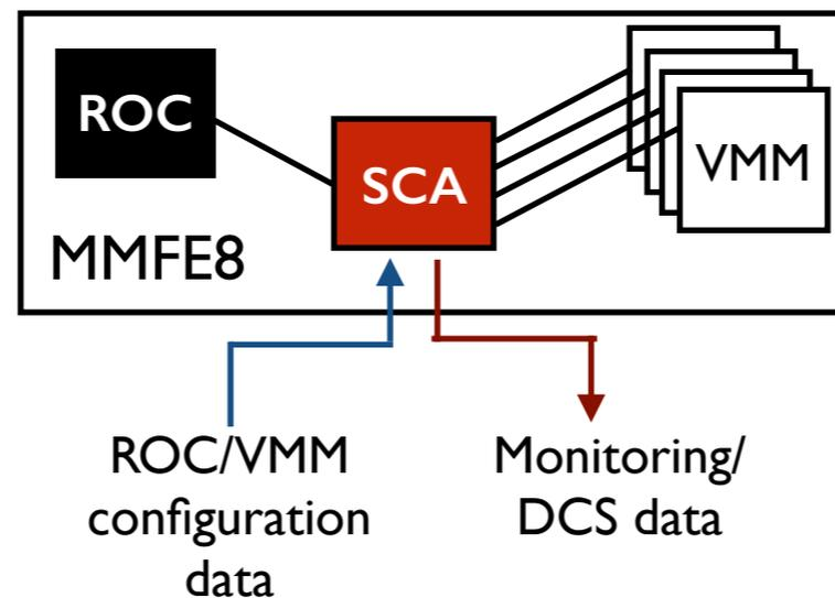
The SCA also samples ADCs and various sensors on the FEBs for **monitoring and detector-control purposes**
