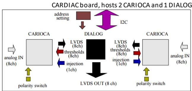
...and one DIALOG chip, which also transmits the data out (LVDS OUT)
