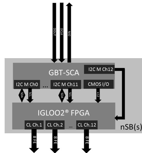
The I2C-bus interfaces are used to communicate with the DIALOG's bus. But the two protocols differs at physical layer...
