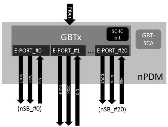
The Electronic Control System data flow in 20 (+1) point-to-point full-duplex e-links.
