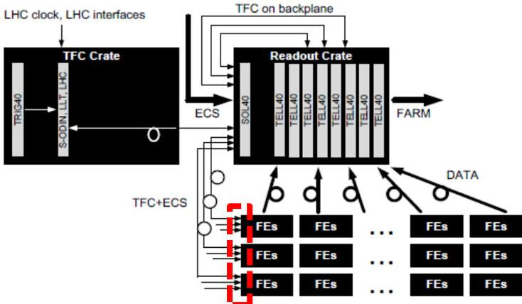
Figure 3: Physical architecture of a partition of the upgraded readout system
