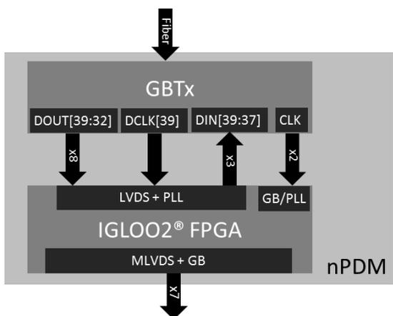
8 (+2) SLVS channels deliver the Timing and Fast Control signals to the FPGA
