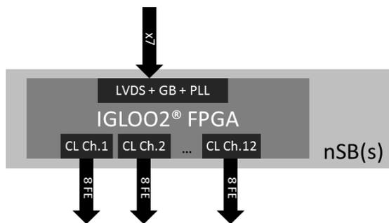
12 FPGA LVDS I/O drivers used to CARDIAC
