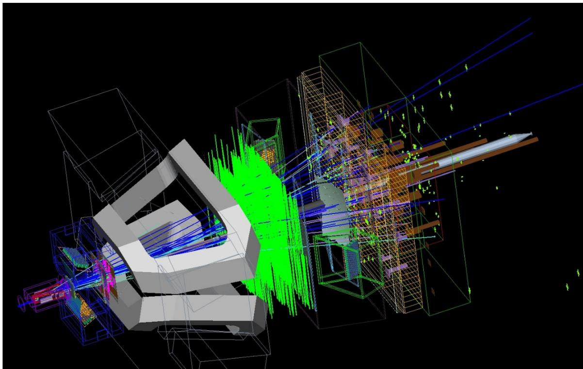
In the upgrade configuration, it comprises 4 stations of MWPC (Multi-Wire Prop. Chamb.) alternated with 4 iron walls
