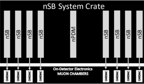
This has required the design of a new Pulse Distribution Module, new Service Board and a new Custom Backplane that fits in the VME 6U crate
