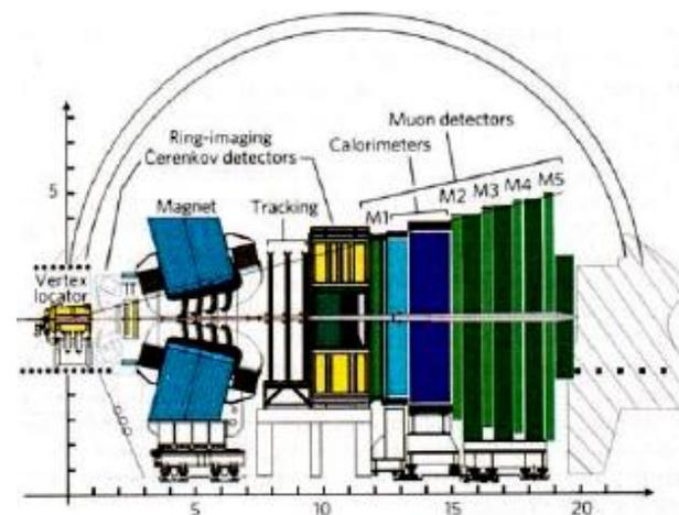
A total amount of 1104 MWPC's are installed in the detector through M1 to M5
