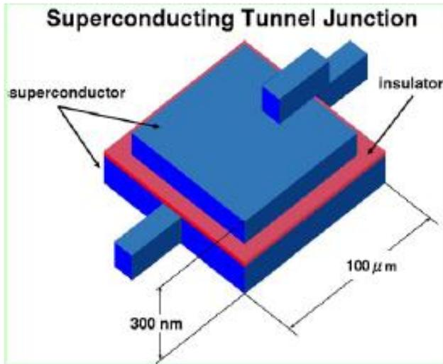
At the superconducting junction, quasi-particles over their energy gap go through tunnel barrier by a tunnel effect. By measuring the tunnel current of quasi-particles excited by an incident particle, we measure the energy of the particle.
