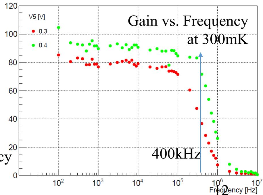
Gain of 80 was achieved for a signal frequency up to 400kHz signals at 300mK.
