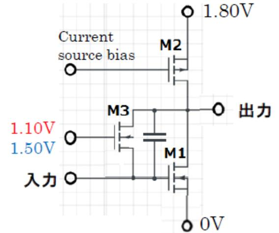
Bandwidth of buffer is enough high for the amplifier of STJ signal (up to 200kHz) both at room temperature and 3K.
