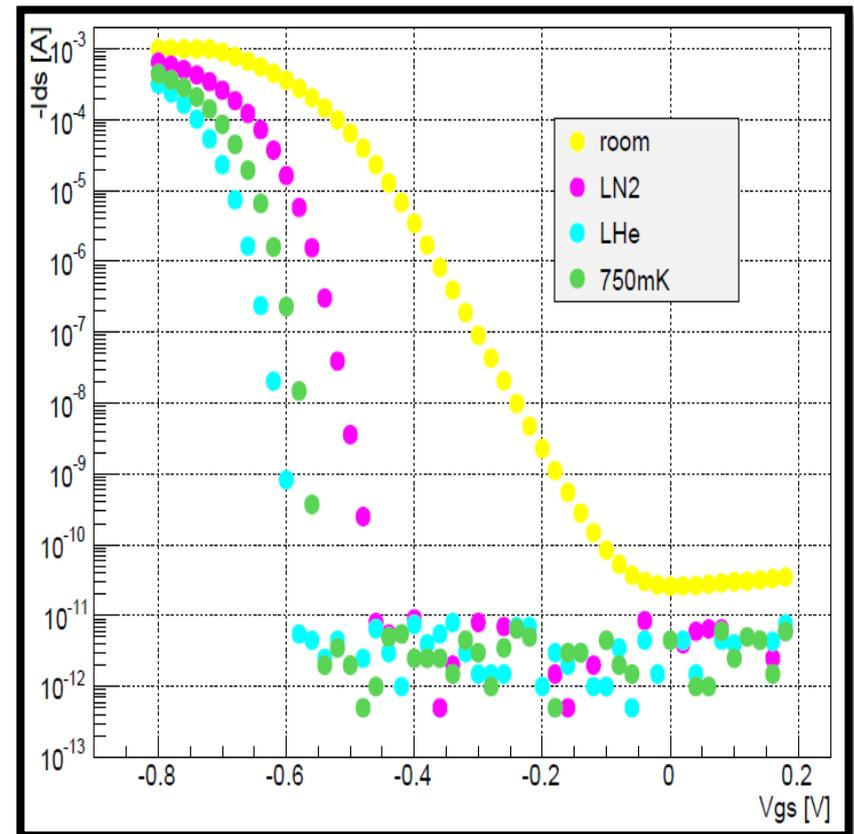
Threshold voltage is changed. But the other properties are almost unchanged.
