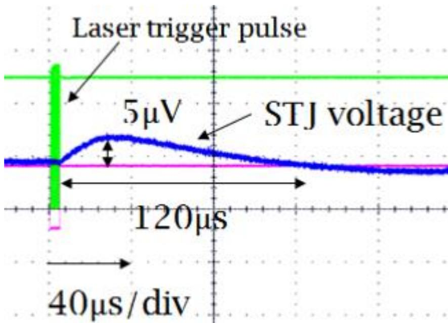
Visible light laser ( $\lambda=465\text{nm}$ ) 10Hz duration
