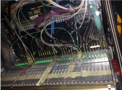
ABBAs in ATCA crate with 10GbE ethernet switch
