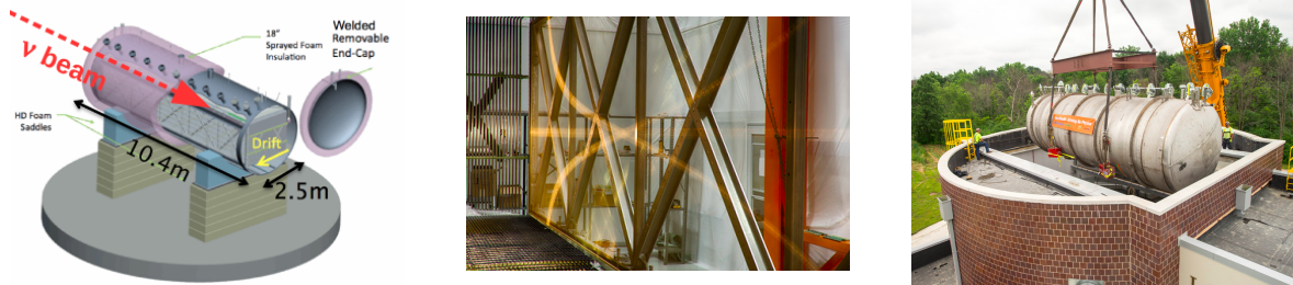
Figure 2 – A schematic of the MicroBooNE detector showing its dimensions with respect to the beam direction (left); a photograph of the wire planes before installation (centre), and a photograph of the assembled TPC plus cryostat being lowered into the Liquid Argon Test Facility (LArTF) (right).
