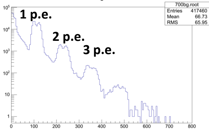
Spectrum of SiPM dark noise
