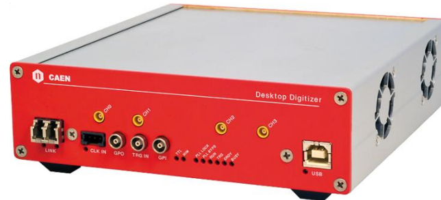
The DT5751 is a 2-4 Channel 10 bit 2/1 GS/s Desktop Waveform Digitizer .
