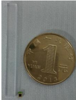
Scintillator strip and SiPM
