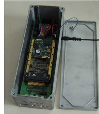
First prototype of DAQ system
